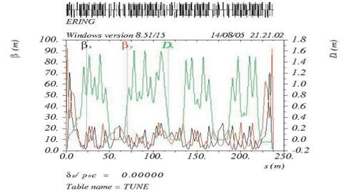
Fig. 1. BEPC II ERING TWISS parameters.
