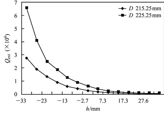
Fig. 7. The distance between the coupler axis and the cavity equator perpendicular bisector impacts the  $Q_{\text{ext}}$ .
