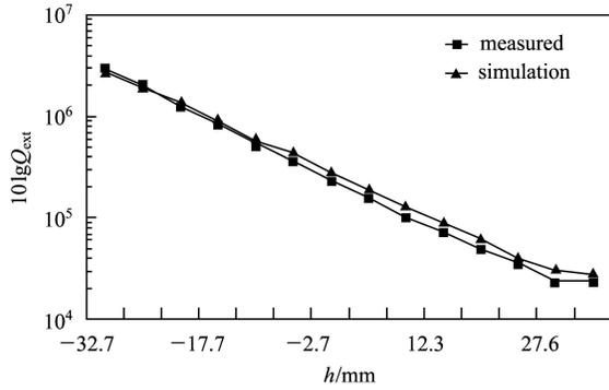
Fig. 4. The simulated  $Q_{\text{ext}}$  and measured  $Q_{\text{ext}}$  for various antenna lengths.
