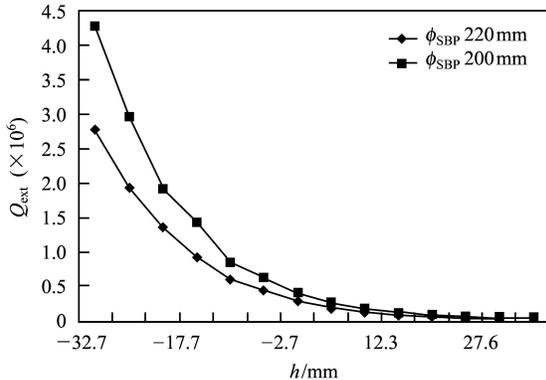
Fig. 6. The diameter of the small beam pipe impacts the  $Q_{\text{ext}}$ .
