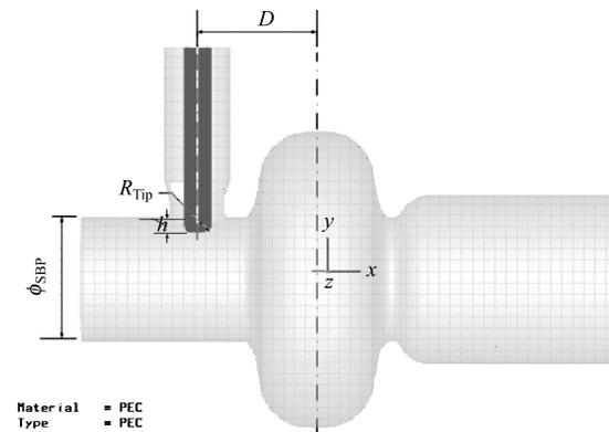
Fig. 3. 1)  $h$  (antenna penetration depth); 2)  $R_{\text{TIP}}$  (the antenna tip radius); 3)  $\phi_{\text{SBP}}$  (the small beam pipe diameter); 4)  $D$  (the distance between the coupler axis and the cavity equator perpendicular bisector).
