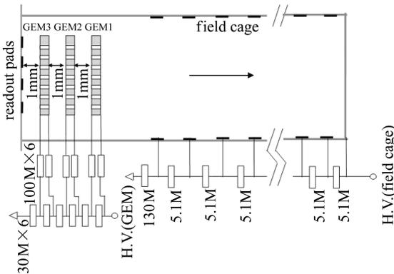
Fig. 2. The high voltage distribution for the field cage and GEM.
