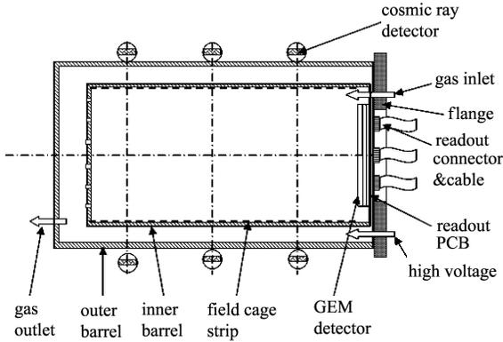
Fig. 1. The scheme of the prototype GEM-TPC.
