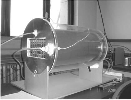
Fig. 3. The photograph of the constructed prototype TPC (electronics is not shown here).
