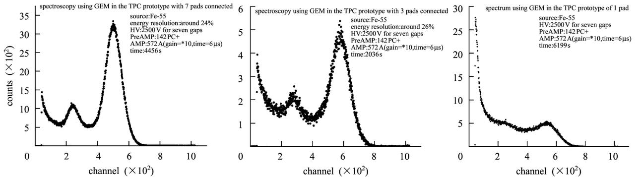
Fig. 4. <sup>55</sup>Fe spectra of GEM used in GEM-TPC prototype with different output pad number.
