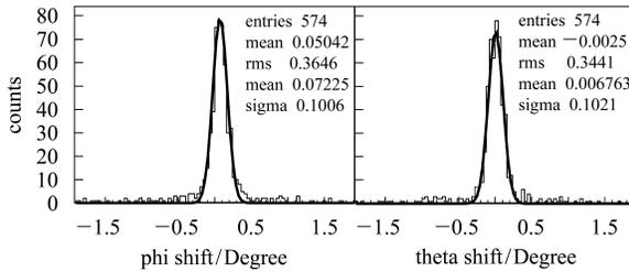
Fig. 1. Azimuthal and polar distribution of the distance between the impact of the propagated track on the PHOS surface and the PHOS cluster position.
