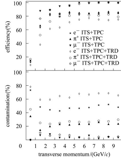
Fig. 3. Track matching efficiency (above) and contamination (down) from TPC to PHOS with different combined barrel detectors, at  $mul.=10$  towards PHOS third module.
