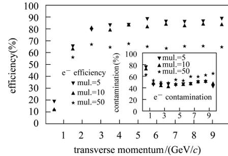
Fig. 4.  $e^-$  track matching efficiency and contamination with different particle multiplicity, in one PHOS module covered by ITS and TPC only.
