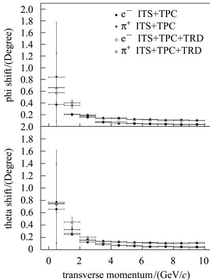
Fig. 2. Mean distance between the track prolongation and the cluster position as a function of the transverse momentum of different particles ( $e^\pm$ ,  $\pi^\pm$ ) and for various configurations of tracking detectors in front of PHOS.
