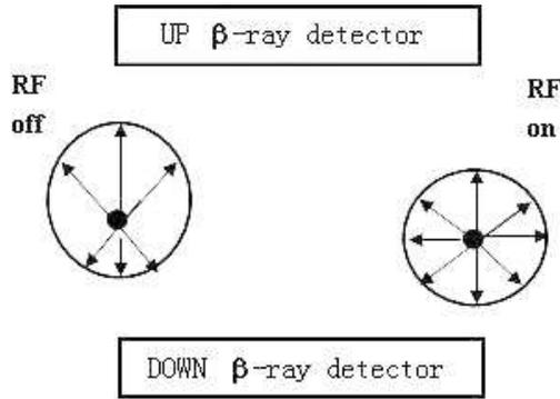
Fig. 1. Angular distribution of  $\beta$ -rays with rf on and off.
