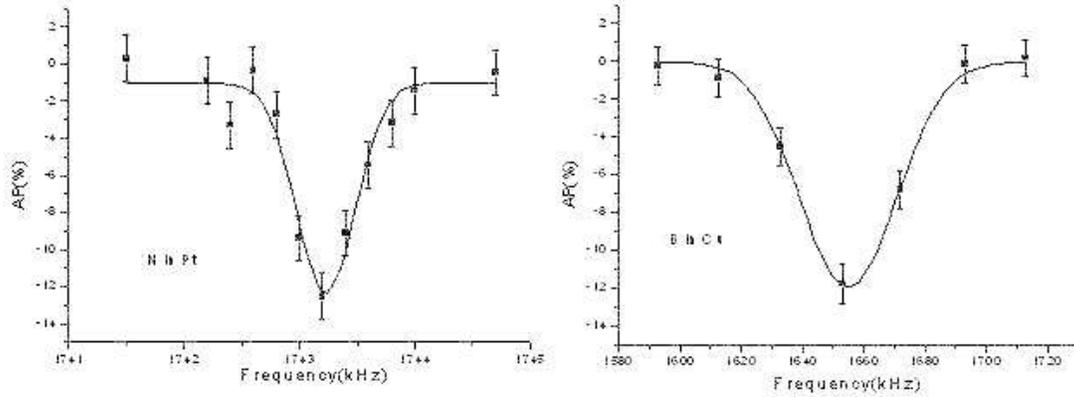
Fig. 2. Typical  $\beta$ -NMR spectra for  $^{12}\text{B}$  and  $^{12}\text{N}$ .
