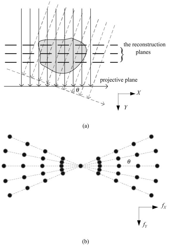
Fig. 1. Tomosynthetic sampling. (a) Schematic illustrations tomosynthesis acquisition; (b) Sampling in Fourier domain of the tomosynthesis acquisition,  $f_X$  and  $f_Y$  are the spatial frequency along the  $X$  and  $Y$  direction, respectively.
