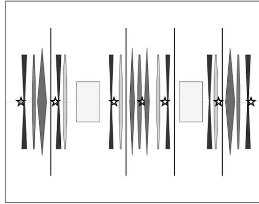
Fig. 2. BPMs (★) of one cell of the SSRF storage ring.
