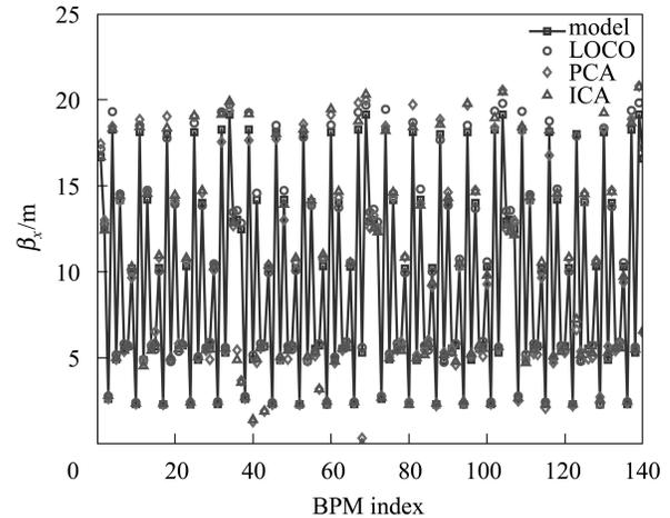
Fig. 6. Comparison of horizontal  $\beta$  functions.
