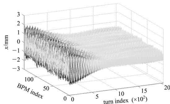
Fig. 1. Typical raw BPM history data after a horizontal kick from an injection kicker.
