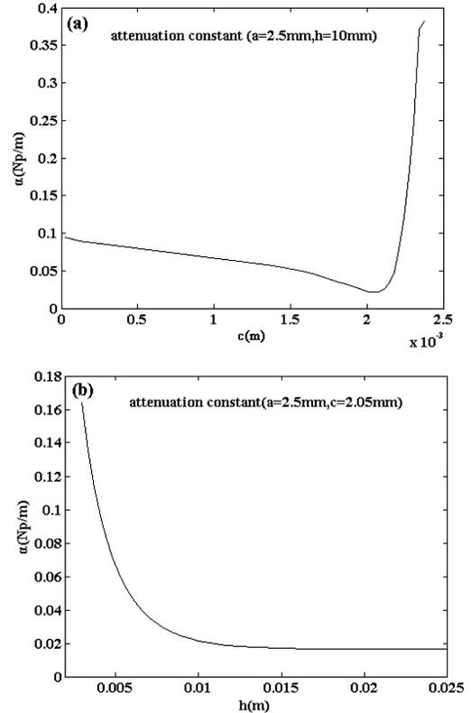
Fig. 4. Calculation of attenuation constant versus (a)  $c$  or (b)  $h$ .
