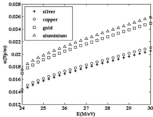
Fig. 6. Calculation of attenuation constant for different materials.
