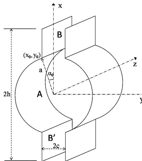
Fig. 1. Schematic of the circular groove guide.
