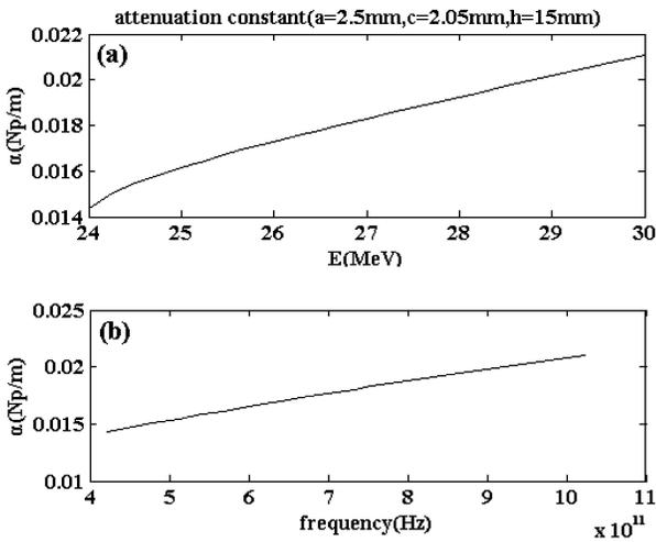
Fig. 5. Calculation of attenuation constant versus (a)  $E$  or (b)  $f$ .
