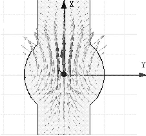
Fig. 2. HFSS simulation shows the distribution of electric field.
