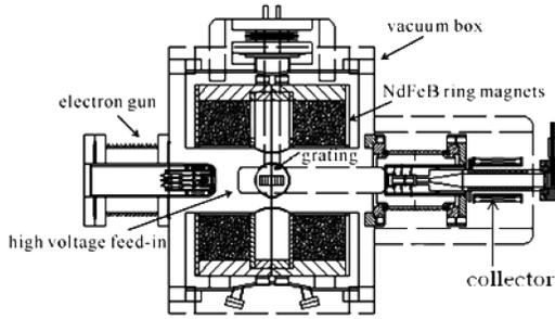
Fig. 2. Set-up of the compact THz source.
