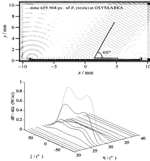
Fig. 5. Simulation and calculation results of SPR. (a) Simulation result of radiation distribution, (b) Calculation of emission power per solid angle.
