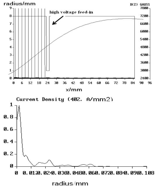
Fig. 4. Dynamic characteristics for electron beam. (a) Longitudinal distribution of e-beam, (b) Radial distribution(normalized current density) at the center of grating.
