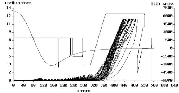
Fig. 6. Simulation of beam dynamics in collector.
