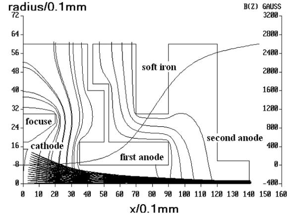
Fig. 3. The structure and electron beam trajectories in the electron gun head. The voltages on the electrodes are optimized for the 35 keV, 200 mA electron beam.
