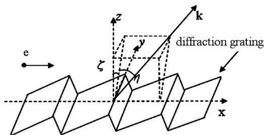
Fig. 1. Schematic of the Smith-Purcell radiation.
