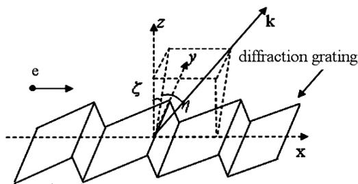
Fig. 1. Schematic of the Smith-Purcell radiation.
