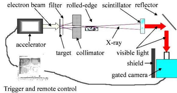
Fig. 12. The time resolved spot size diagnostic.
