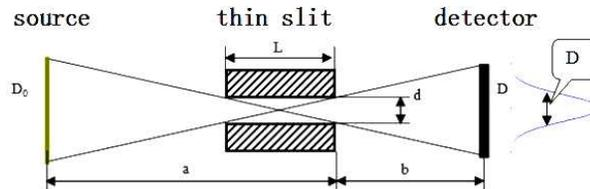
Fig. 1. The sketch of spot size diagnostic.
