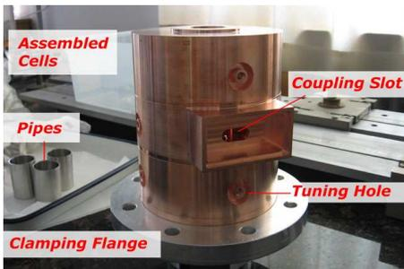
Fig. 1. Cavity in assembling showing the coupling slot.
