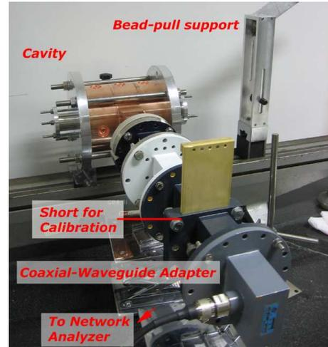
Fig. 2. Assembled cavity in microwave measurement.
