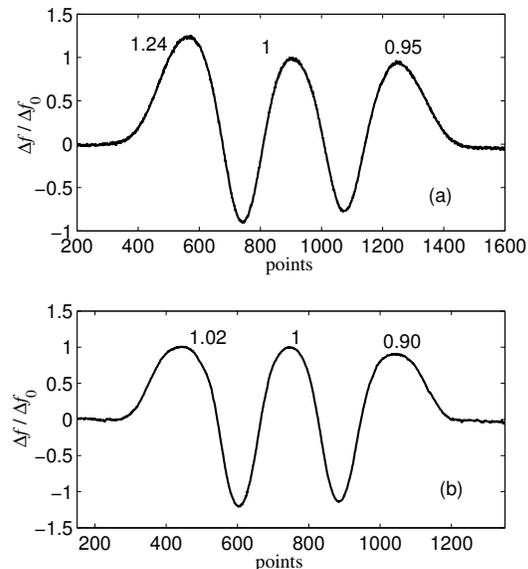
Fig. 3. On-axis field distribution of Cavity- I (a) and Cavity- II (b) measured by ‘‘bead-pull’’ method.
