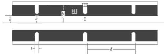
Fig. 1. Sketch of regular accelerator cavities. In the figure, Region I is vacuum; Region II is ceramic with dielectric constant  $\epsilon_r$ ; Region III is copper.  $a$  is the iris radius,  $b$  is the outer radius, and  $h$  is the beam hole radius.  $t$  is the thickness of the iris, and  $d$  is the length of one cell.
