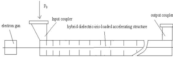
Fig. 2. Sketch of compact accelerator.
