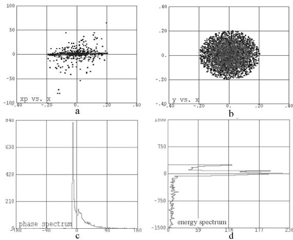
Fig. 5. Beam spectra at the exit of the accelerating tube. (a)  $x'-x$  (mrad-cm); (b)  $x-y$  (cm-cm); (c) Phase spectrum (degree-particle numbers); (d) Energy spectrum (particle numbers-keV).
