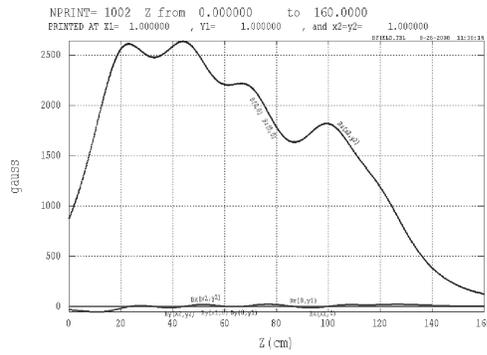
Fig. 4. Magnetic field distribution of focus coils along the linac.
