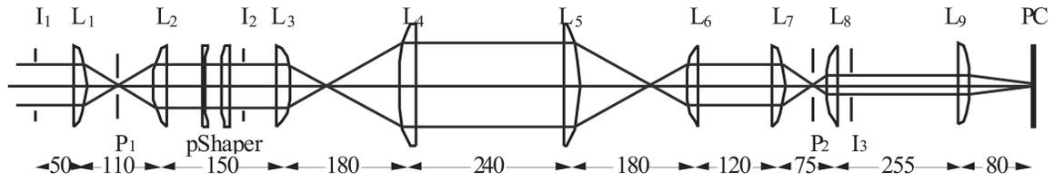
Fig. 2. Schematic of transport beam line for the photocathode.
