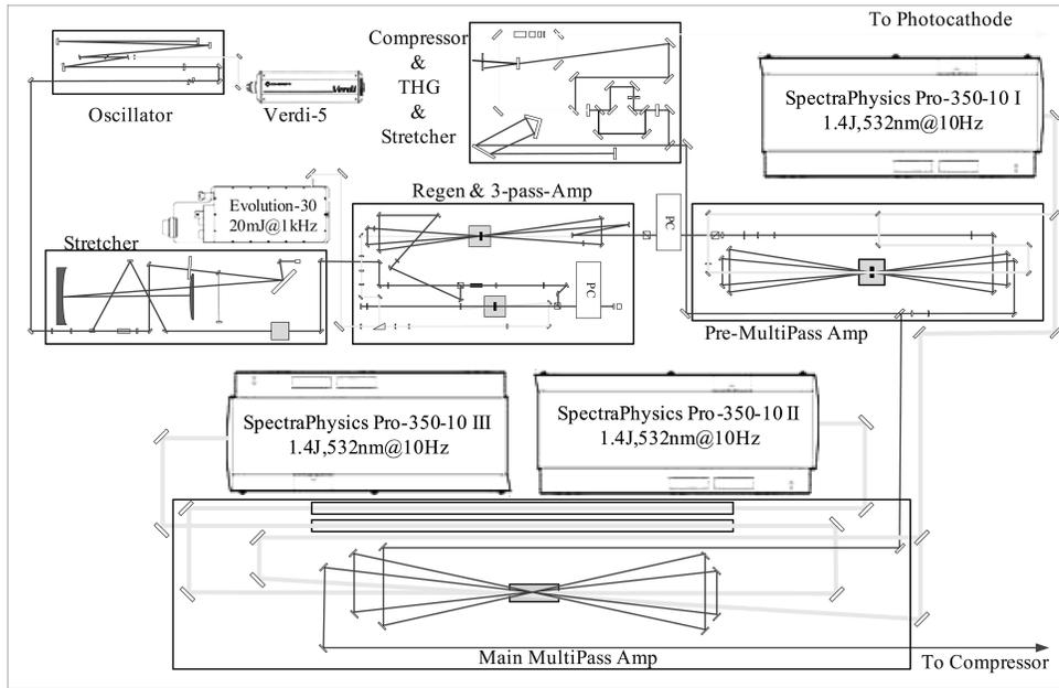
Fig. 1. Layout of the TW laser system.
