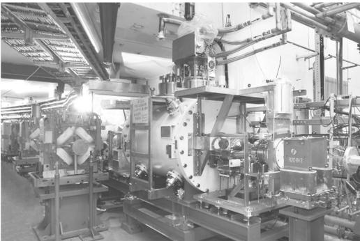
Fig. 3. A superconducting cavity in installation.
