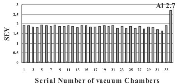
Fig. 4. Measured SEY of TiN-coated chambers.
