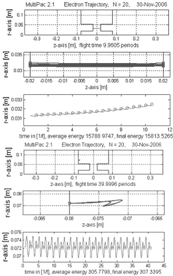
Fig. 2. Results of 2D simulation in pill-box cavity. The upper three figures show the two points multipacting at the nose and the lower three figures show the one point multipacting effect on the wall.
