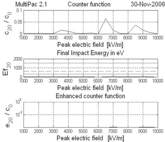
Fig. 3. Results of the SSRF SHB cavity. On the top is the counter function, in the middle is the final impact energy of the electron and on the bottom is the enhanced counter function. The figures show no multipacting, because the enhanced counter function is negligible in this field region.
