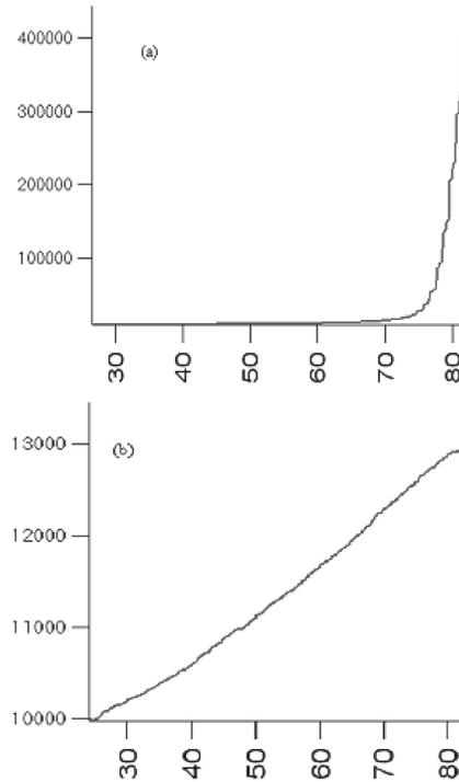
Fig. 4. Multiplication of 10000 randomly distributed electrons, the field  $E_{acc} = 0.021$  MV/m, (a) the focusing coils are turned on, and (b) the focusing coils are turned off.
