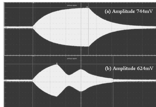
Fig. 1. Pick up signal from coupler. (a) Power supplies are off; (b) Power supplies are on.
