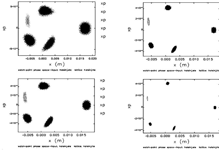
Fig. 2. Particle tracking for the injected beams. Left up: 50 nm-rad, left down: 20 nm-rad, right up: 5 nm-rad, right down: 1 nm-rad.
