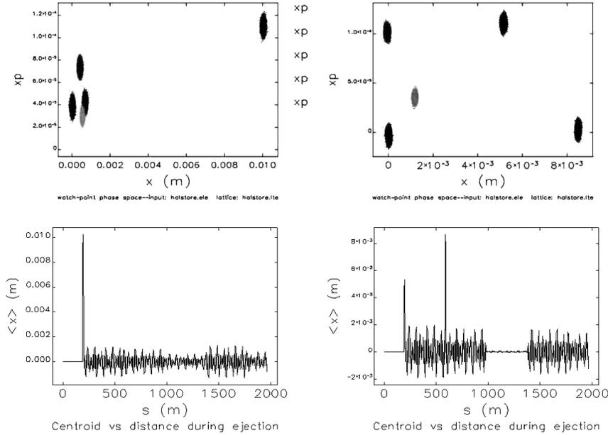
Fig. 4. The tracking results of stored beam in and after injection with errors, the left and the right are the phase space (up) and the central trajectory (down) of different stored bunches.
