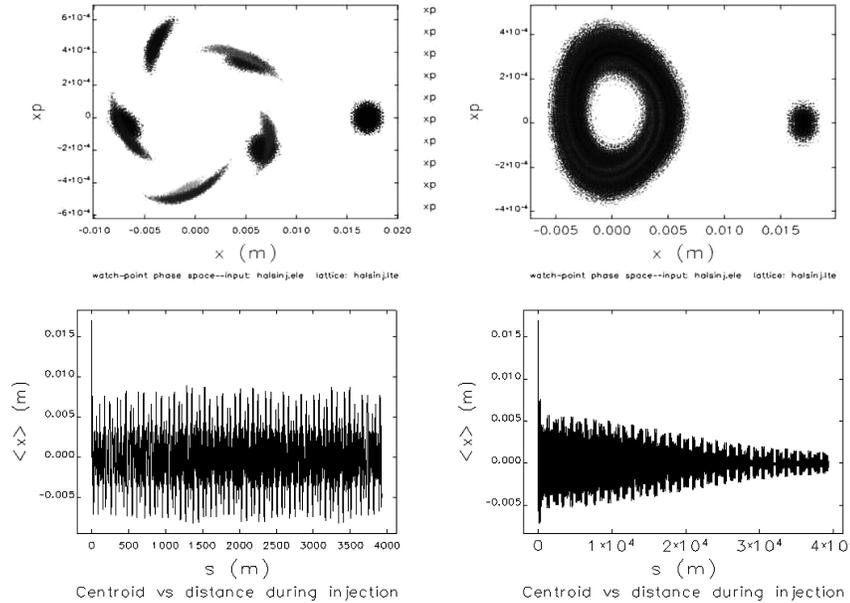
Fig. 3. Particle tracking for the injected beams. Left: 5 turns tracking, right: 50 turns, up: phase space, down: central trajectory.
