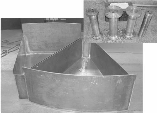
Fig. 8. The 44.45 MHz RF cavity under construction.
