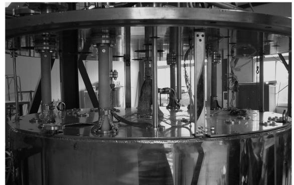
Fig. 16. The cryostat for the QWR cavity.
