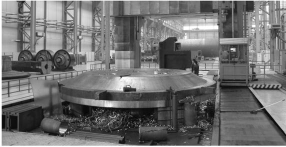
Fig. 5. The top/bottom yokes under machining.
