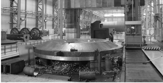
Fig. 5. The top/bottom yokes under machining.
