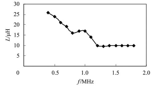
Fig. 2. The total inductance dependence of the RF frequency.
