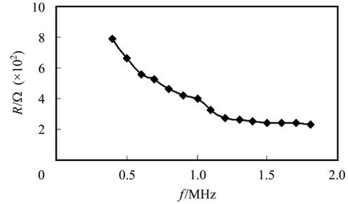
Fig. 1. The shunt impedance dependence of the RF frequency.
