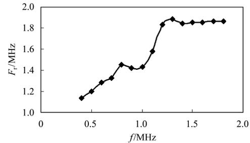
Fig. 4. The resonant frequency dependence of the RF frequency.
