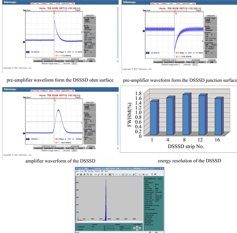
Fig. 2. Testing results for the DSSSD.
