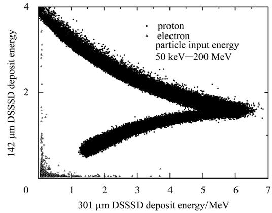
Fig. 3. Energy deposition of different energies of electrons and protons in the  $\Delta E$ -E Si detectors.
