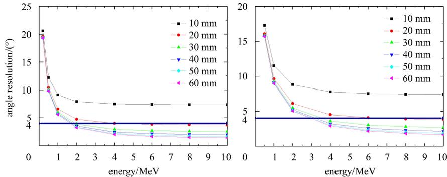
Fig. 6. The calculated results for the detector angle resolution under different conditions (thickness on the left is 60  $\mu\text{m}$ , and on the right is 150  $\mu\text{m}$ ).
