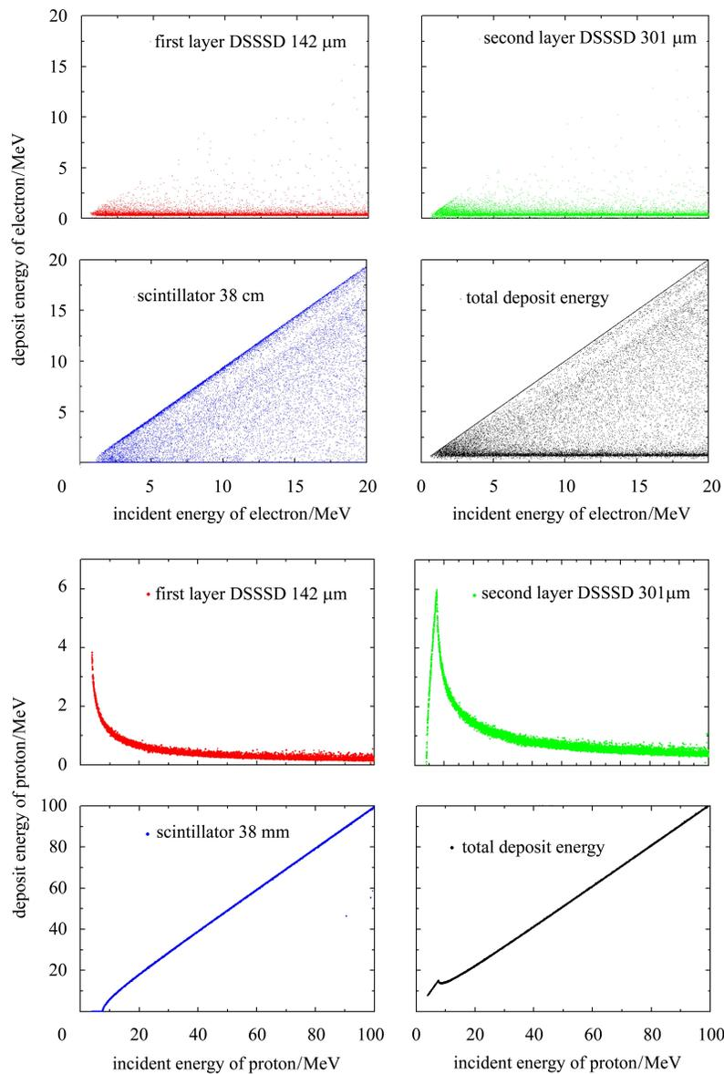
Fig. 4. The deposit energy vs. incident energy of electrons and protons in each layer of the detector and the total energy.
