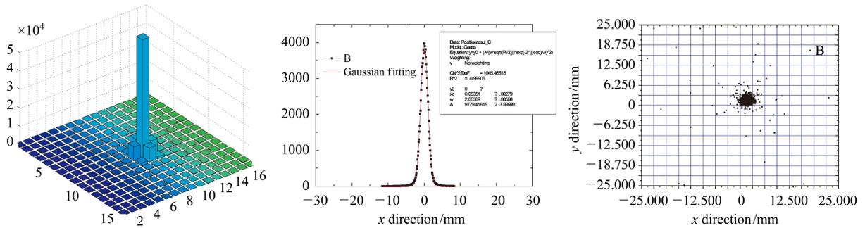
Fig. 5. Incident electron in the detector's position resolution simulation results.
