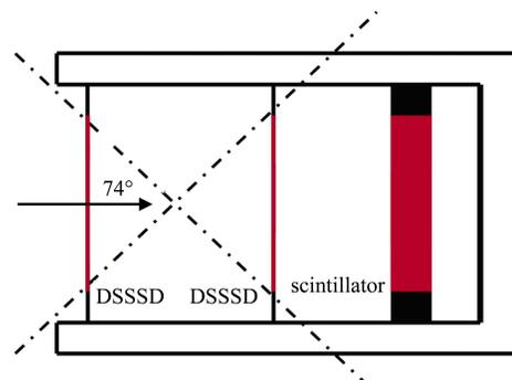
Fig. 1. The structure of the position-sensitive charged particle detector.
