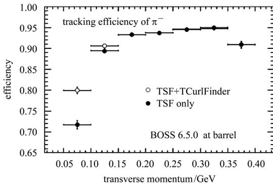
Fig. 10. A comparison of tracking efficiency of TSF only and TSF plus TCurlFinder in  $\psi' \rightarrow \pi^+\pi^-J/\psi$ ,  $J/\psi \rightarrow 1^+1^-$  using real data.
