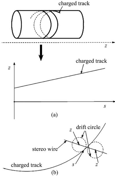
Fig. 3. (a) A helix in 3D transforms into a straight line in the  $s$ - $z$  plane; (b) stereo hits are selected using the information of the drift circle and parameters of the charged track.
