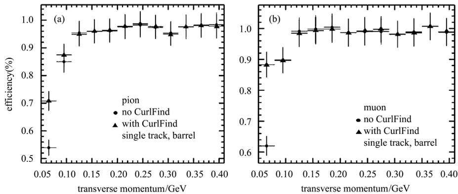
Fig. 6. (a) Comparison of tracking efficiency of Monte Carlo data of single  $\pi^-$ . (b) Comparison of the tracking efficiency of Monte Carlo data of single  $\mu^-$ .
