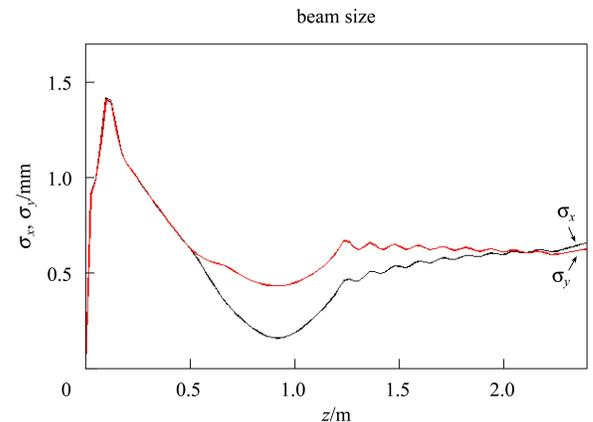
Fig. 8. Rms beam envelope along the distance.
