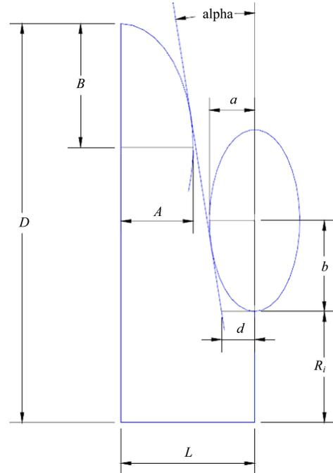
Fig. 5. Typical parameters of half SC cell.
