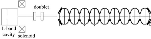
Fig. 2. Basic setup of the photocathode RF injector.
