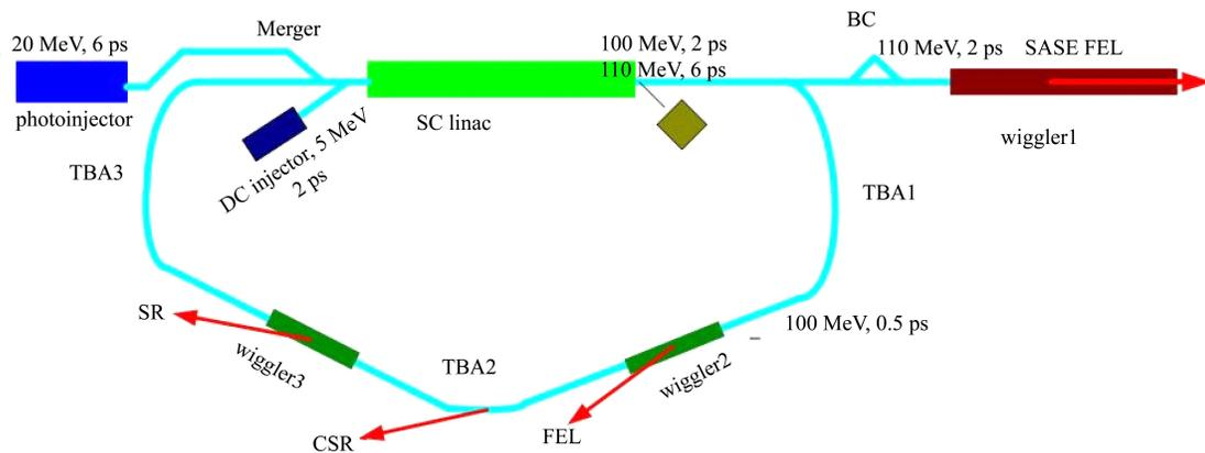
Fig. 1. Scheme of the ERL-FEL test facility.
