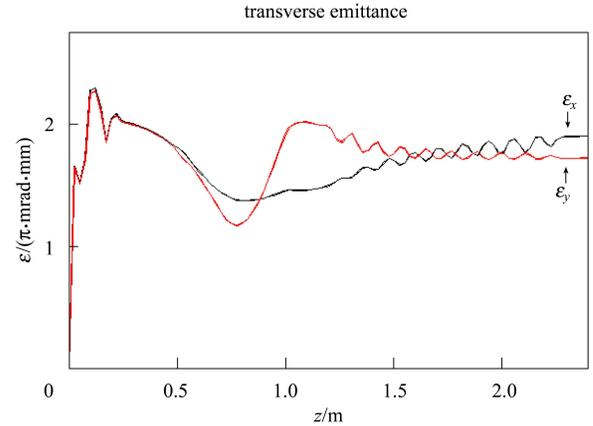
Fig. 7. Normalized emittance evolution along the distance.
