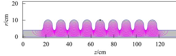
Fig. 4. Electric field of the 9-cell cavity.
