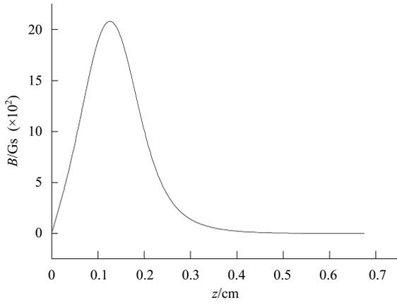
Fig. 6. The typical solenoid focusing field.
