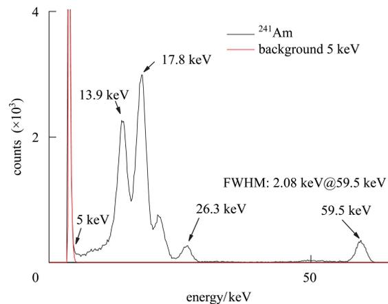
Fig. 11. The  $^{241}\text{Am}$  spectrum obtained by a single Si-PIN detector with an area of 10 mm  $\times$  10 mm and thickness of 1 mm. The measurement was done at  $-5^\circ\text{C}$ .
