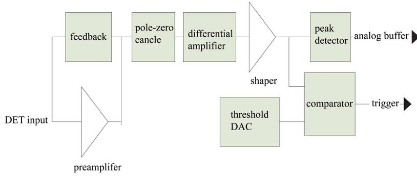
Fig. 1. A simplified block diagram for one channel of the RENA-3 ASIC.
