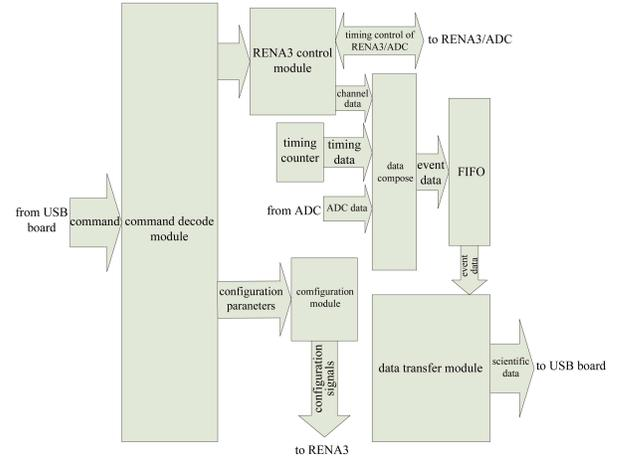
Fig. 5. A logic diagram of the FPGA on the DAQ mother board.
