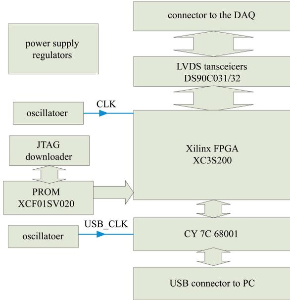
Fig. 7. A block diagram of the USB board.
