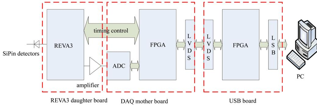
Fig. 2. The block diagram of the whole ME prototype.
