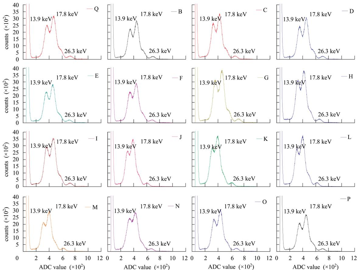
Fig. 10. 16  $^{241}\text{Am}$  spectra measured simultaneously by the prototype of the ME readout system at room temperature.
