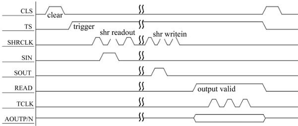
Fig. 6. The timing control of RENA-3.
