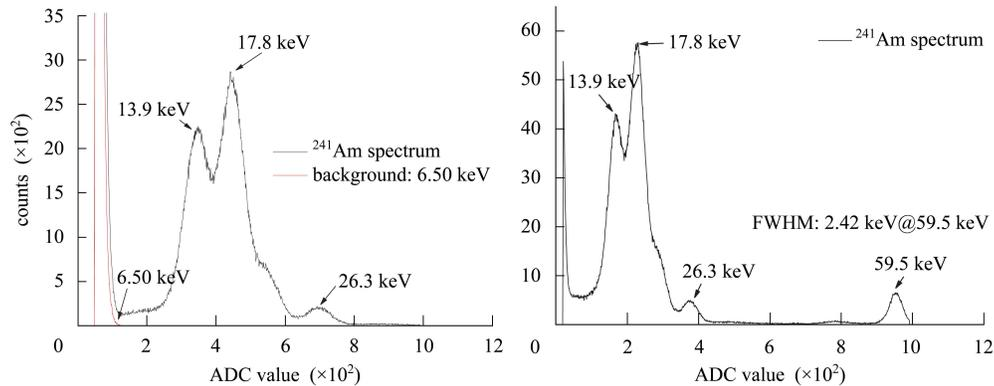
Fig. 9. The  $^{241}\text{Am}$  spectra measured by a single Si-PIN detector at room temperature. The area and thickness of the detector are 10 mm  $\times$  10 mm and 1 mm respectively.
