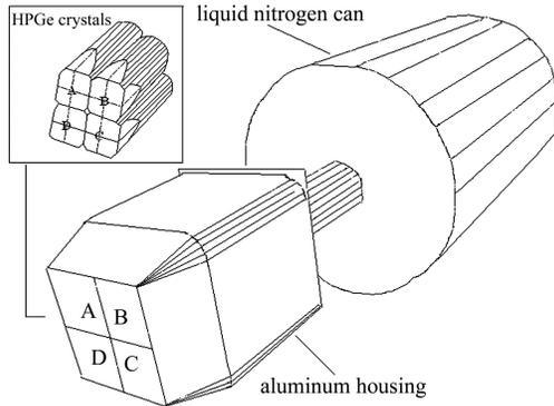
Fig. 1. Schematic view of the geometrical arrangement of HPGe crystals in a segmented Clover detector.
