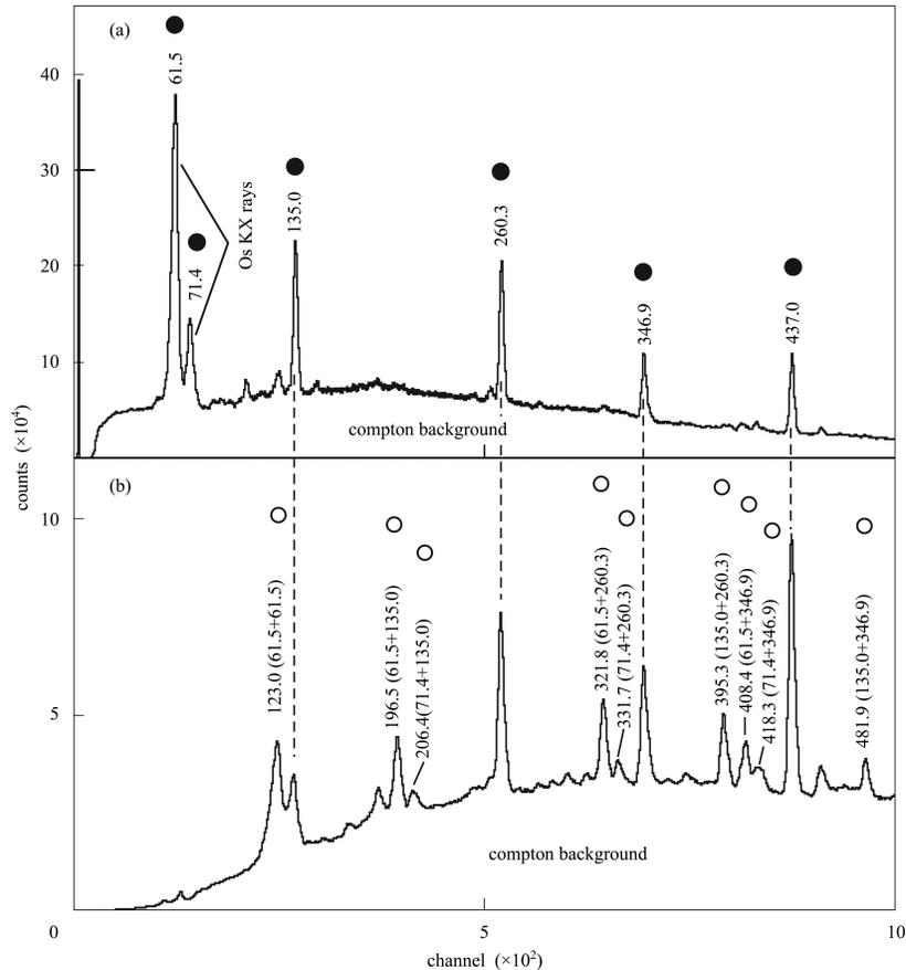
Fig. 3. Summing effects of photo peaks in a Clover detector. (a) Single spectrum of A crystal, (b) add-back spectrum of A and B. Solid and open circles correspond to photo peaks and sum peaks, respectively.
