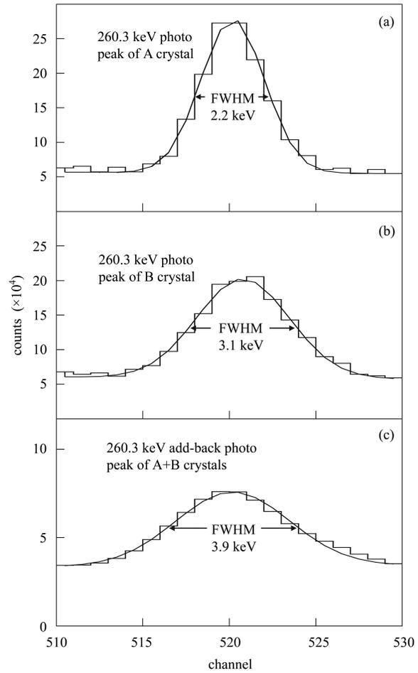
Fig. 2. A typical resolution of the 260.3 keV photo peak from  $^{176}\text{Ir}$  decay obtained in single mode and add-back mode.
