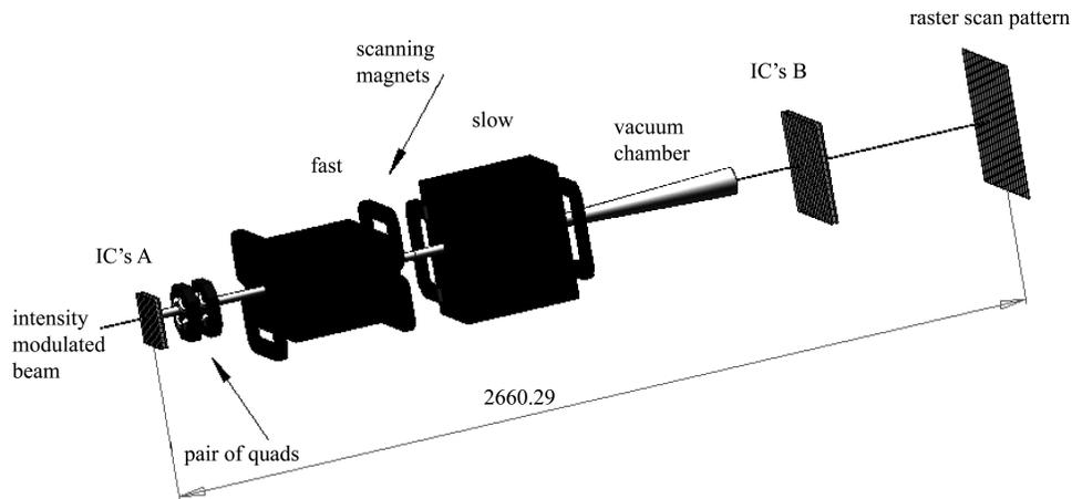
Fig. 4. Scheme of the pencil beam nozzle for APTF.
