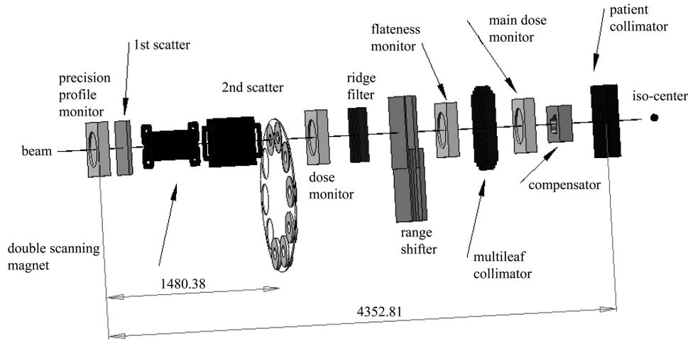
Fig. 1. Scheme of the beam spreading nozzle for the APTF.
