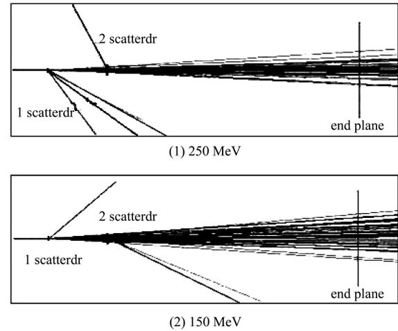
Fig. 2. Trajectories of 50 particles with the two scatterers at 150 MeV and 250 MeV.
