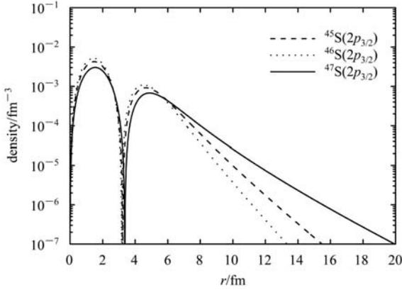
Fig. 1. The density distributions for the  $2p_{3/2}$  states in  $^{45}\text{S}$ ,  $^{46}\text{S}$  and  $^{47}\text{S}$ . The dashed, dotted and solid curves are the density distributions of the last neutron in  $^{45}\text{S}$ ,  $^{46}\text{S}$  and  $^{47}\text{S}$ , respectively.
