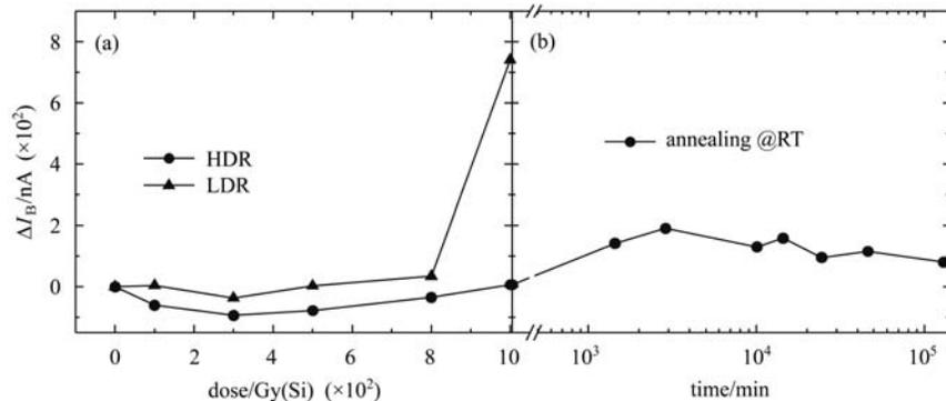
Fig. 2. The radiation response (a) and annealing behavior (b) of excess base current of the B type transistors.
