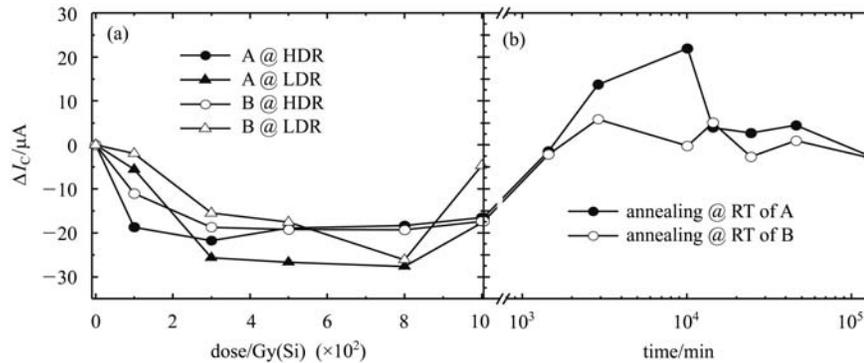
Fig. 4. Radiation response (a) and annealing behavior (b) of collector current of the A and B type transistors.
