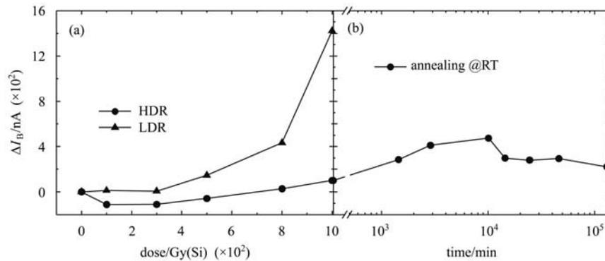
Fig. 1. The radiation response (a) and annealing behavior (b) of excess base current of the A type transistors.
