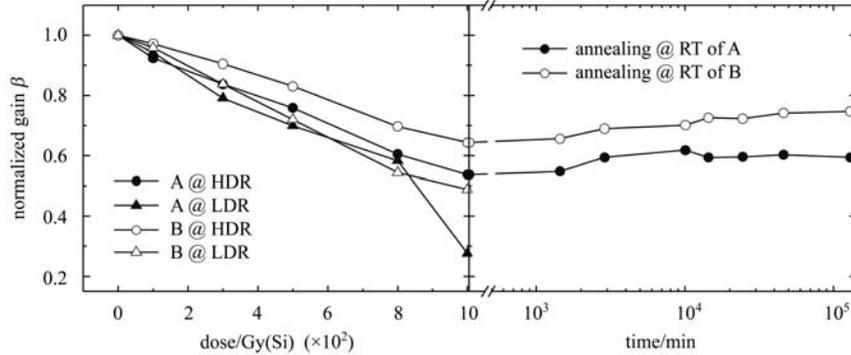
Fig. 3. Radiation response and annealing behavior of normalized current gain of the A and B type transistors.
