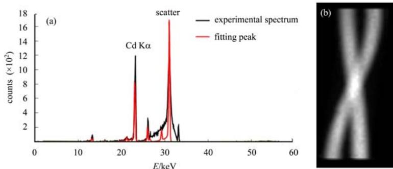
Fig. 2. (a) A typical X-ray spectrum measured from the test sample by the HPGe detector. (color online) (b) Tomographic data (sinogram) from the test sample for Cd K $\alpha$  ( $E_{K\alpha} = 23.17$  keV).
