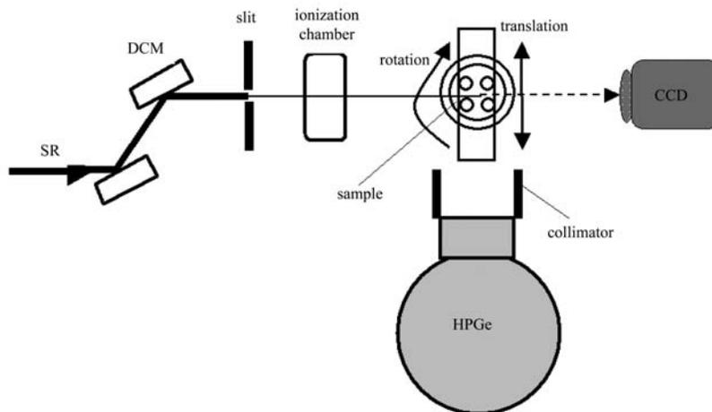
Fig. 1. Schematic diagram of the XFCT.
