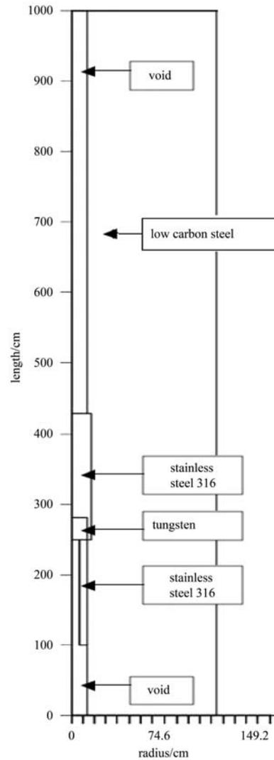
Fig. 3. The shutter neutron beam stop model.
