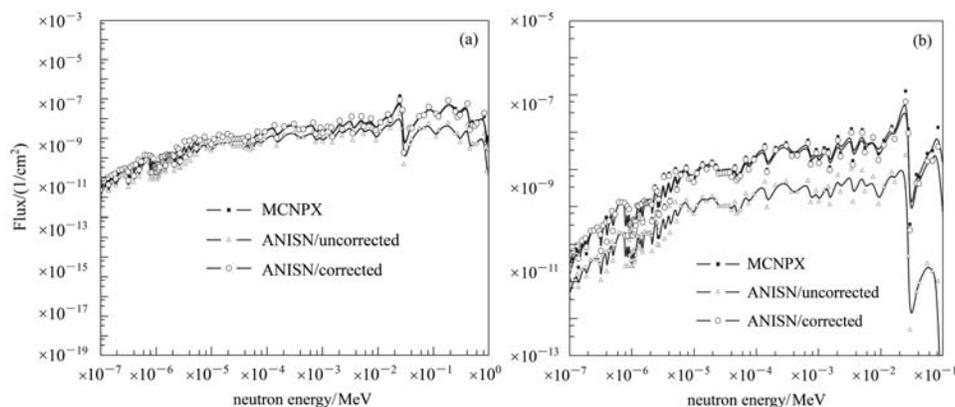
Fig. 2. The neutron fluxes calculated by MCNPX, ANISN/uncorrected cross section and ANISN/corrected cross section.
