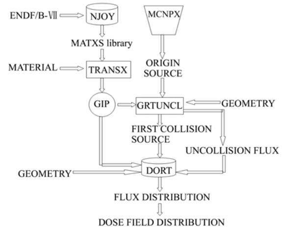
Fig. 1. The calculation flow diagram for shielding analyses.
