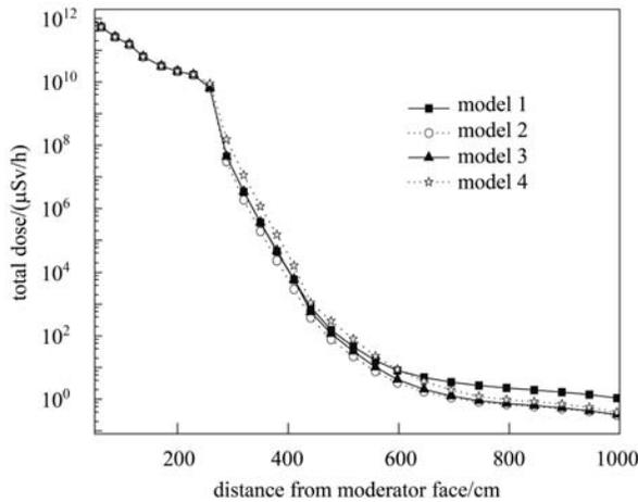
Fig. 5. The total dose axial distributions of four models.
