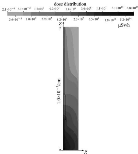
Fig. 4. The isodose contours of stainless steel 316 shutter neutron beam stop.
