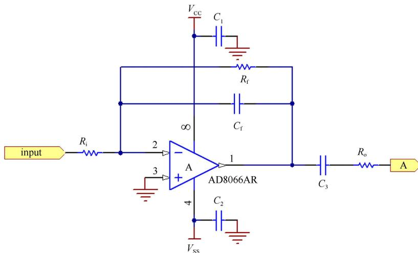
Fig. 3. The pre-amplification circuit.
