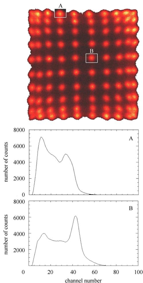
Fig. 9. The measured responses of the detector module with a  $12\times 12$  LYSO crystal array using  $^{137}\text{Cs}$  source. Top: the measured raw flood image; Middle: the measured energy spectrum from a crystal element in the edge of the detector; Bottom: the measured energy spectrum from a crystal element in the center region of the detector.
