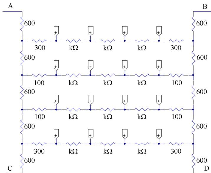
Fig. 2. The resistor-chain network of the readout circuit.
