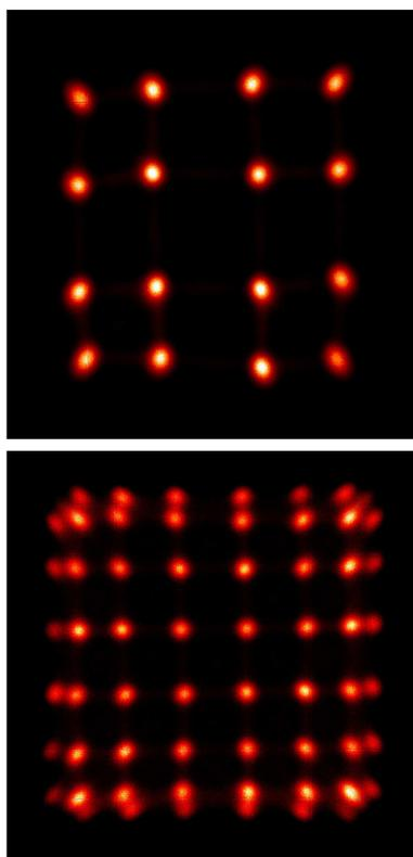
Fig. 8. The measured raw flood images of the detector module with two LYSO crystal arrays using  $^{137}\text{Cs}$  source. Top: with a  $4\times 4$  crystal array; Bottom: with a  $8\times 8$  crystal array.
