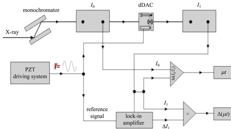
Fig. 2. The pattern of measuring modulated EXAFS. The PZT driving system generates a sine wave as the input signal of the PZT actuators in dDAC and the Lock-in Amplifier. The modulated absorption signals are extracted by the Lock-in Amplifier.
