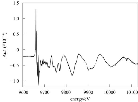
Fig. 3. Experimental results of the modulated EXAFS at Zn K edge. The initial pressure in dDAC was 5 GPa, and a 10 Hz sine wave was used.
