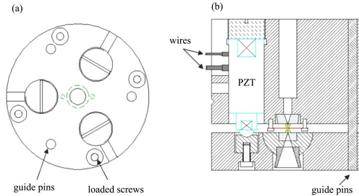
Fig. 1. A schematic diagram of dDAC: three piezo actuators (PZT) are installed between two parts of the cell and controlled by a PZT driving system. The pressure on the sample will change with the motion of the PZT. (a) End-on view; (b) Cross-sectional view.
