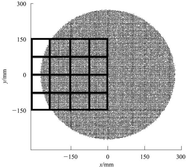
Fig. 4. The position distribution of scattered  $^{12}\text{C}$  on the MWPC and the CsI detectors. The circle and the square correspond to the distribution on the MWPC and the CsI detectors, respectively.
