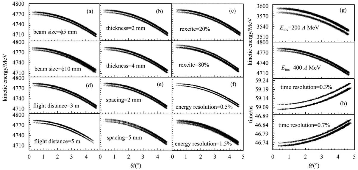
Fig. 3. The relation between scattering angles (from  $0^\circ$  to  $5^\circ$ ) and scattering kinetic energy with different variable parameters which correspond to (a) beam size, (b) target thickness, (c) excited ratio of the excited state with 4.4 MeV, (d) flight distance, (e) wire spacing of the MWPC, (f) energy resolution of the CsI detectors, (g) incident kinetic energy, besides (h) for the relation between scattering angles and TOF with time resolution of the plastic scintillators.
