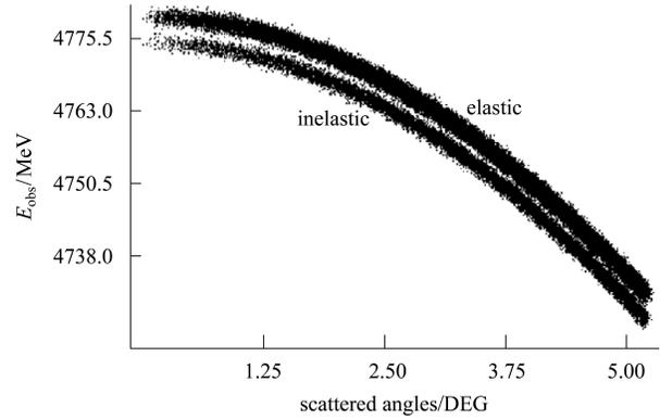
Fig. 2. Relation between the scattering angles  $\theta$  and the actual detected kinetic energy  $E_{\text{obs}}$ .
