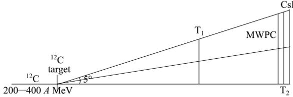
Fig. 1. The schematic of the experimental setup for 200-400 A MeV  $^{12}\text{C}+^{12}\text{C}$  system.
