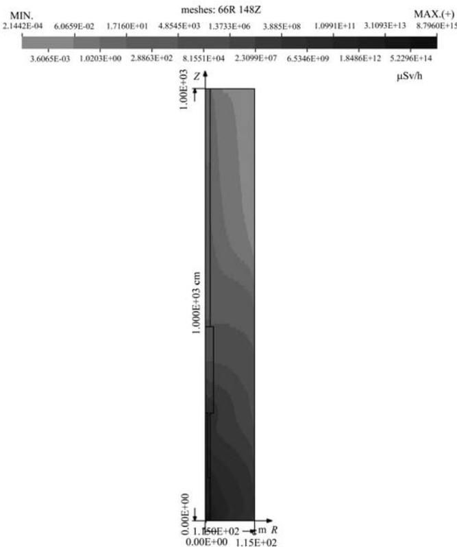
Fig. 6. The isodose contours of 316 stainless steel shutter neutron beam stop.
