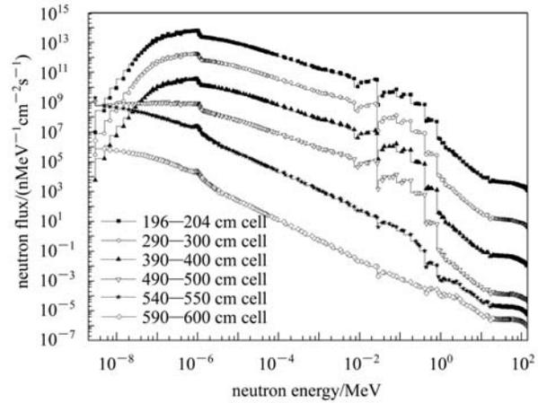
Fig. 5. The neutron flux density energy spectra for the calculation model.
