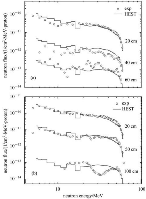
Fig. 2. Calculated neutron flux for iron (a) and concrete (b) slabs vs. experimental results.
