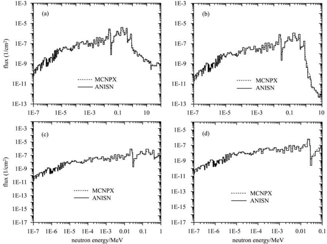
Fig. 4. Neutron flux calculated by ANISN and MCNPX with different sources, (a) 100, (b) 10, (c) 1 and (d) 0.1 MeV.
