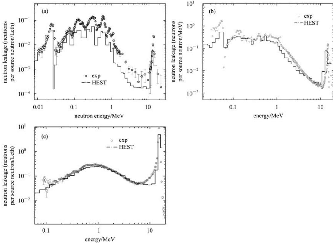
Fig. 3. Calculated neutron leakage in (a) iron, (b) nickel and (c) tungsten spheres vs. experimental results.
