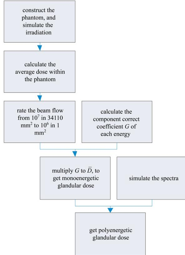
Fig. 3. Flow chart of the glandular dose simulation in DBCT.
