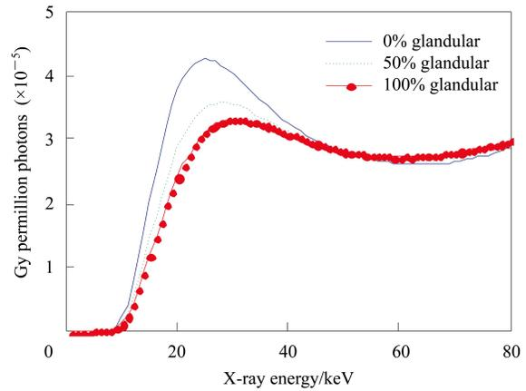
Fig. 7. The graph shows a monoenergetic glandular dose as a function of incident X-ray energy for 0%, 50%, and 100% glandular tissue.
