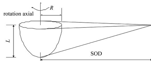
Fig. 1. The diagram shows the geometry used for Monte Carlo simulations.  $R$ =radius of the cross-section circle,  $L$ = the height of half ellipsoid, SOD=source-to-object distance.
