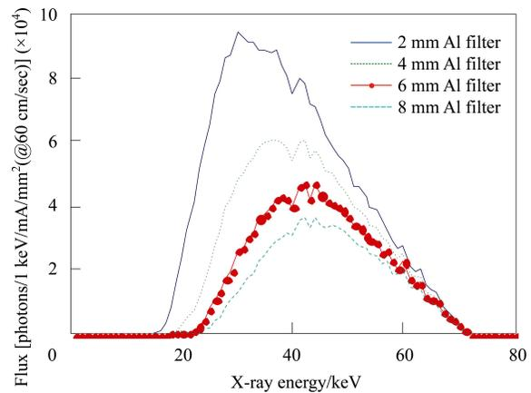
Fig. 8. The X-ray spectra  $\Phi(E)$  of the W anode simulated with same 70 kV voltage and Al filters of different thicknesses.
