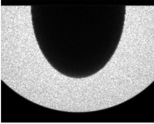
Fig. 2. Projection of an  $R=6.5$  cm,  $L=10$  cm phantom. SOD=60 cm, detector-to-object distance is 10 cm, with the upper edge of the detector 10 cm higher than the horizontal plan.
