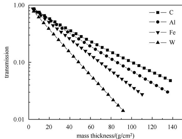
Fig. 2. The transmission curves of X-ray under the narrow beam condition.
