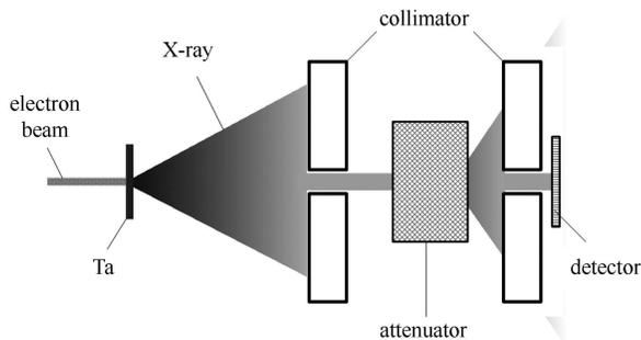
Fig. 1. Simulation model of the experimental setup for X-ray attenuation measurement.
