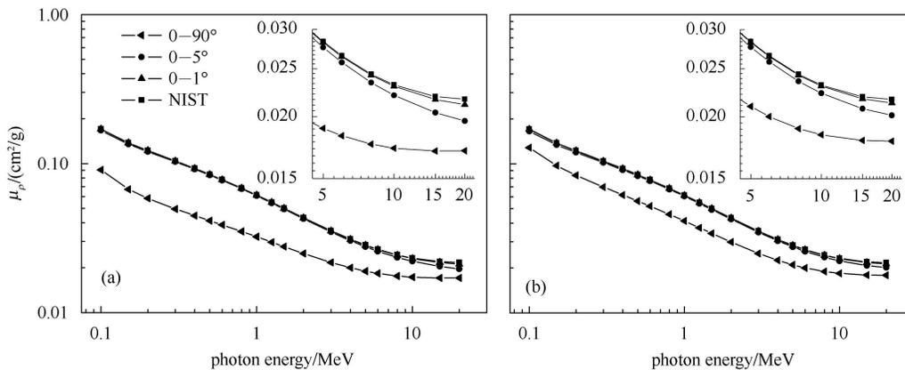
Fig. 5. Comparison of calculated mass attenuation coefficients of aluminum within various emergence angle intervals of transmitted photons. The thickness of aluminum is 1 cm for (a) and 20 cm for (b).
