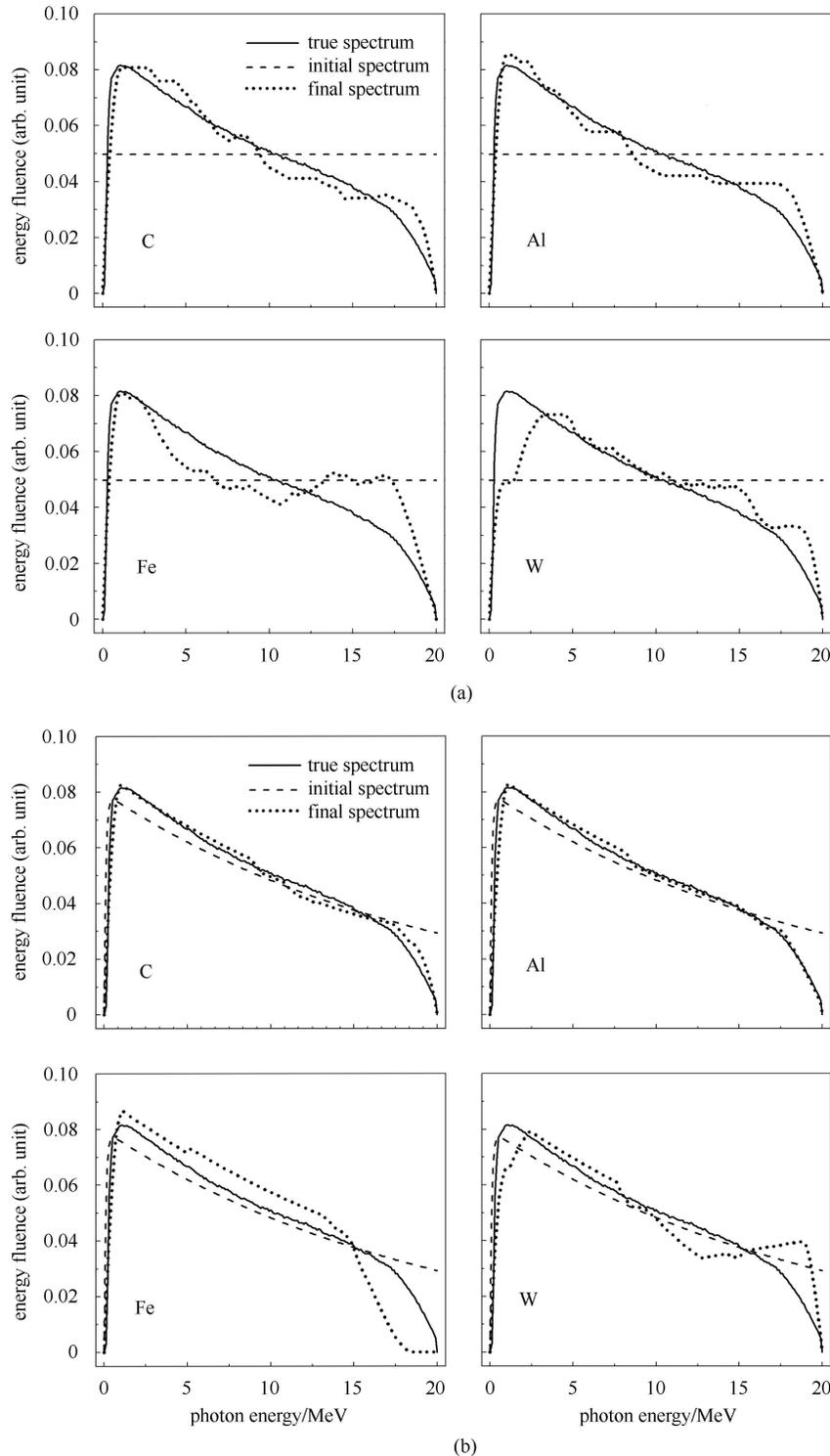
Fig. 3. Reconstruction of X-ray spectra with different filter materials. (a) Pre-spectrum of uniform distribution; (b) Pre-spectrum of pulsefunction distribution.
