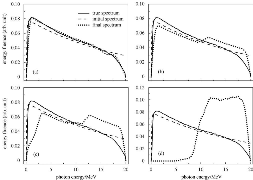
Fig. 6. Reconstructed X-ray spectra from transmission data containing photon energies within different emergence angle intervals. (a)  $0-1^\circ$ ; (b)  $0-5^\circ$ ; (c)  $0-10^\circ$ ; (d)  $0-90^\circ$ .
