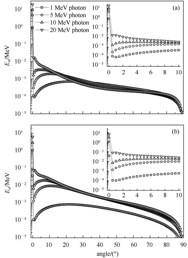
Fig. 4. Angular distribution of monoenergetic photons transmitted through aluminum. The thickness of aluminum is 1 cm for (a) and 20 cm for (b).  $E_{at}$  is the average transmission energy.
