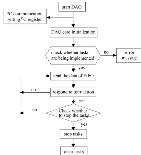
Fig. 4. Program flow chart for the DAQ software.
