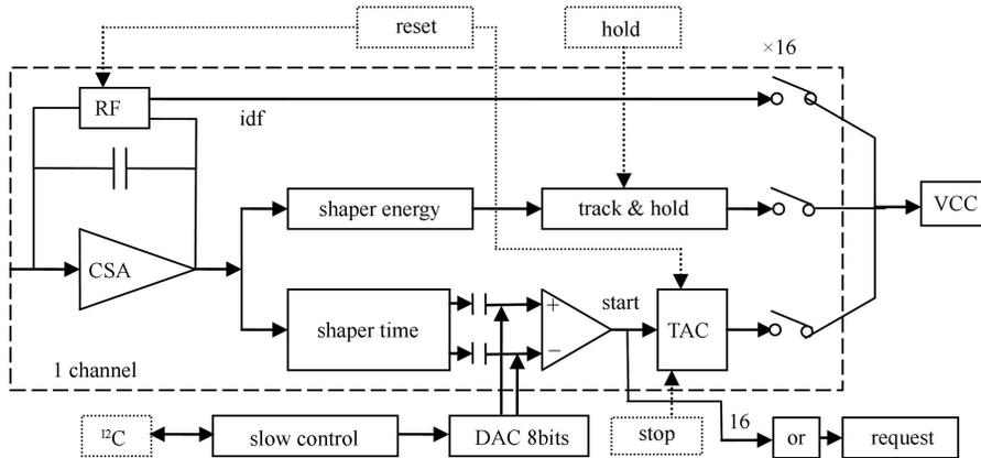
Fig. 2. One channel schematic diagram of ATHED.
