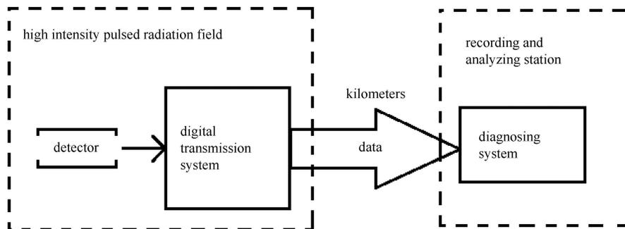
Fig. 1. The digital transmission system.
