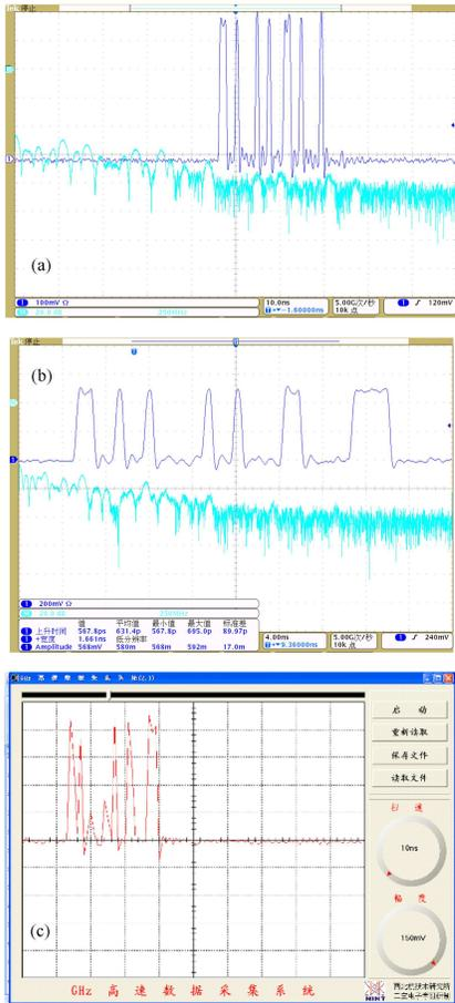
Fig. 10. (color online) Test for valid signal distinguishing. (a) The input signal #1 (all pulsed widths <math>< 3\text{ ns}</math>, the sampling is not triggered); (b) The input signal #2 (one pulsed width >math>> 3\text{ ns}</math>); (c) The sampling result for #2.
