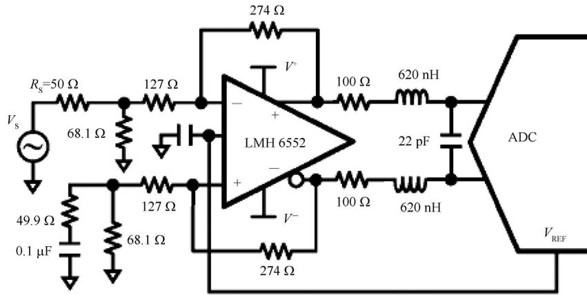
Fig. 3. The single-to-difference conversion circuit.
