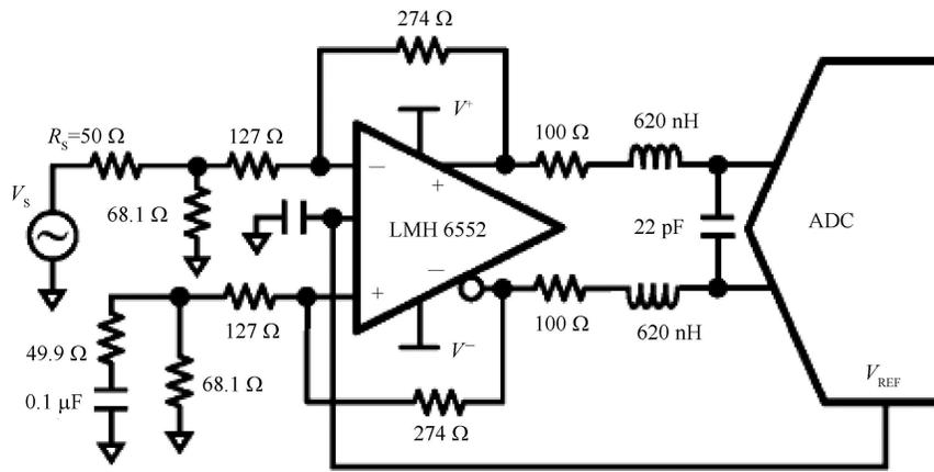
Fig. 3. The single-to-difference conversion circuit.
