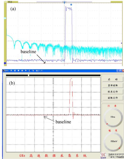
Fig. 11. (color online) Test for the baseline restoration. (a) The input signal (50 mV baseline drift); (b) Sampling result.
