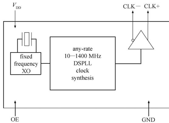
Fig. 4. The clock source circuit.
