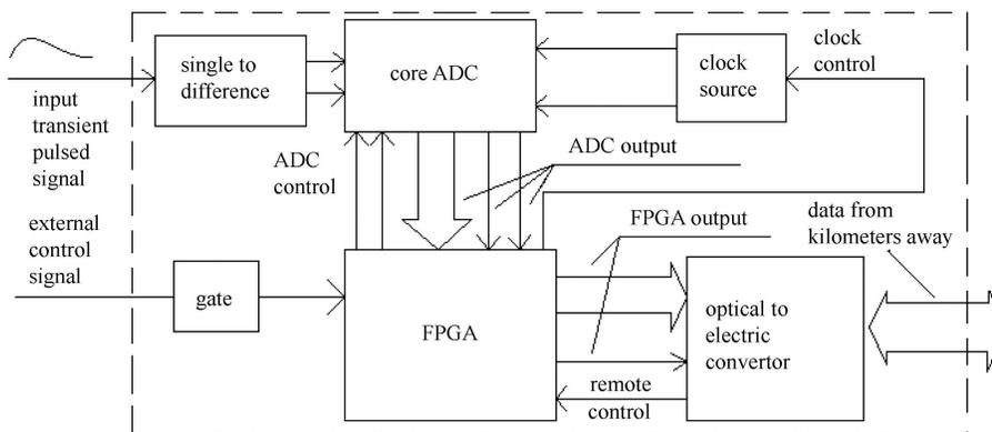
Fig. 2. The simplified measuring system circuit.
