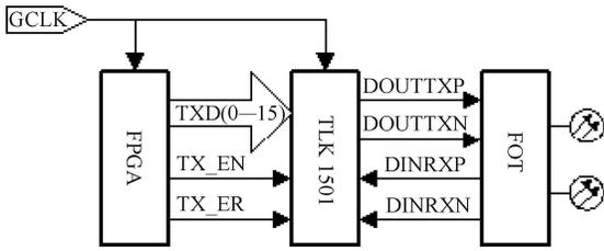
Fig. 6. The circuit of parallel/serial and electrical/optical conversion.
