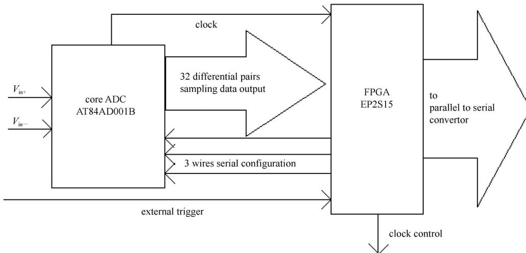
Fig. 5. The circuit with ADC and FPGA.
