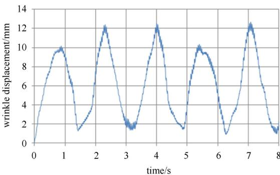
Fig. 7. The wrinkle vibration of the foil.
