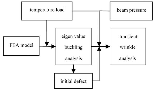
Fig. 4. The foil wrinkle analysis flow chart.
