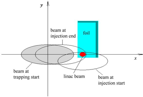
Fig. 1. The injection painting process of CSNS [6].
