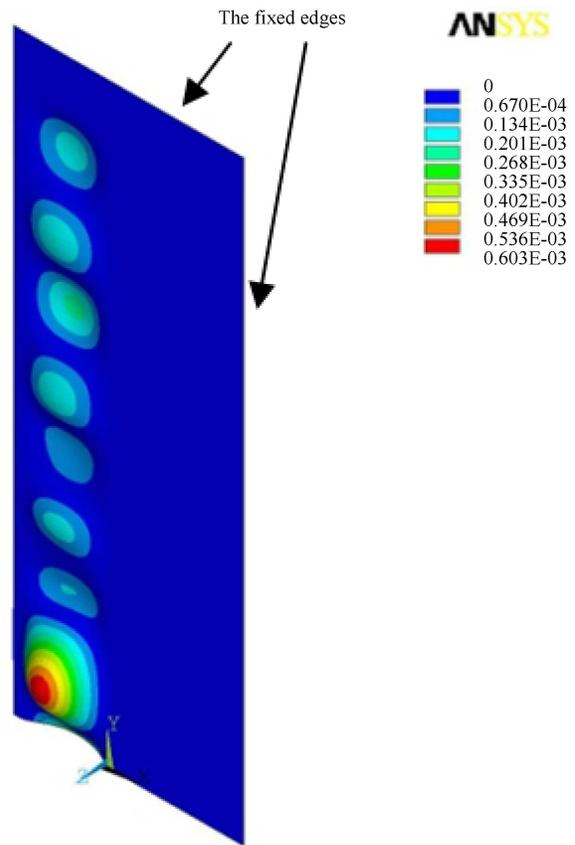
Fig. 12. The maximum wrinkle shape of installing carbon fibers scheme.
