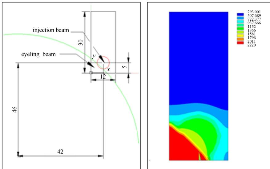
Fig. 5. The loads of wrinkle analysis for SNS. (L: The beam conditions of SNS; R: The foil's temperature distribution for SNS).
