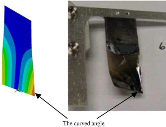
Fig. 6. The comparison of wrinkle shape between the simulation and the reality of SNS.
