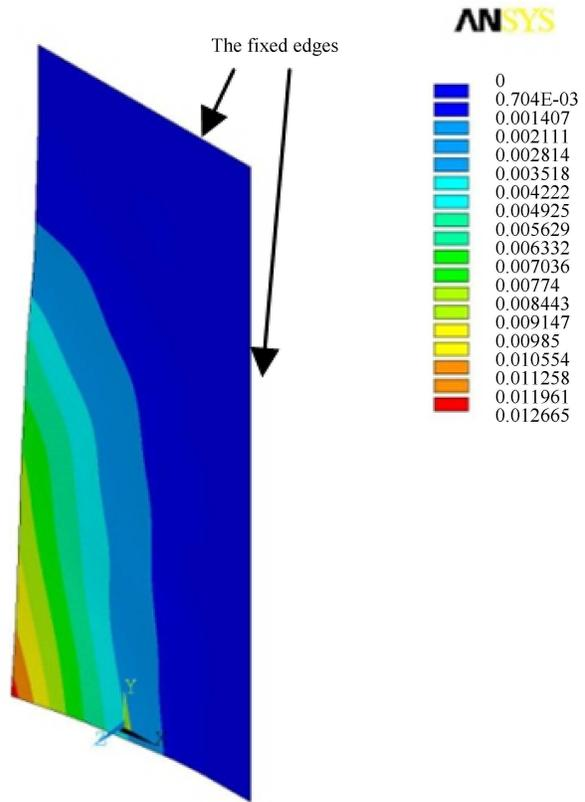
Fig. 8. The maximum wrinkle shape of the foil.
