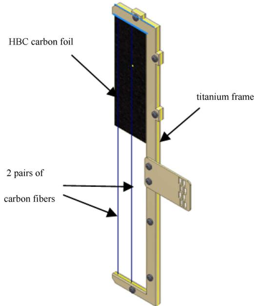
Fig. 13. The preliminary design of mounting scheme for CSNS.
