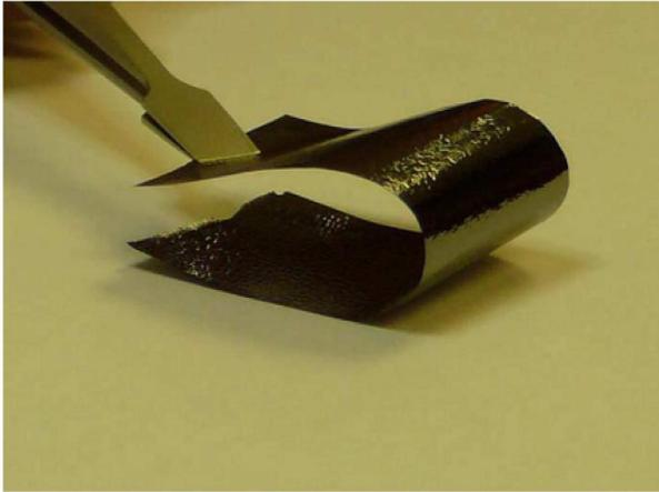
Fig. 9. The new type of HBC foils [7].
