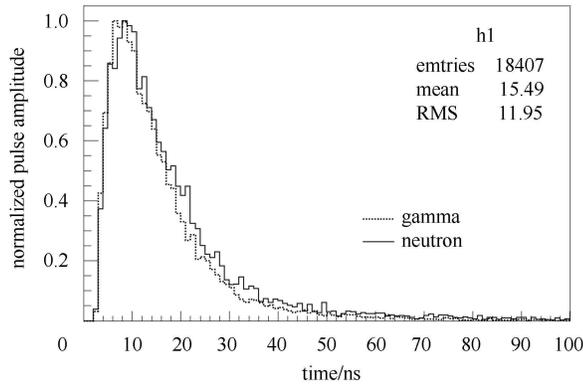
Fig. 8. Light pulse waveform comparison of neutron and gamma in one PMT (Normalized amplitude).
