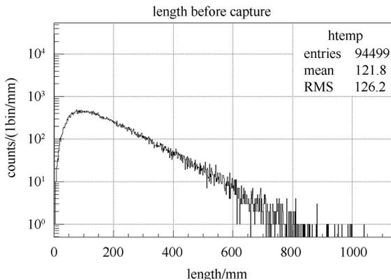
Fig. 5. Distance distribution of the n-p collision and (Gd, n) capture.
