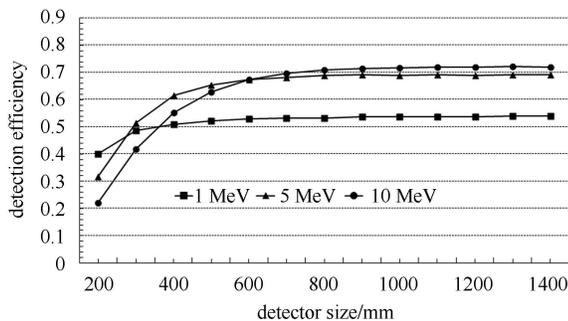
Fig. 2. Detection efficiencies of cube detectors of different sizes.
