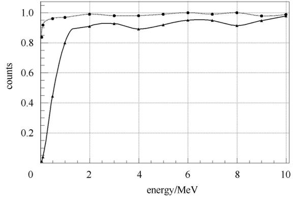
Fig. 11. Count rate of neutrons at different energy; the solid line is the relative count ratio of the far-end of detector, the dotted line is the one of near-end.
