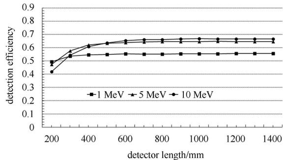
Fig. 3. Detection efficiencies of cylinder detectors with different lengths.
