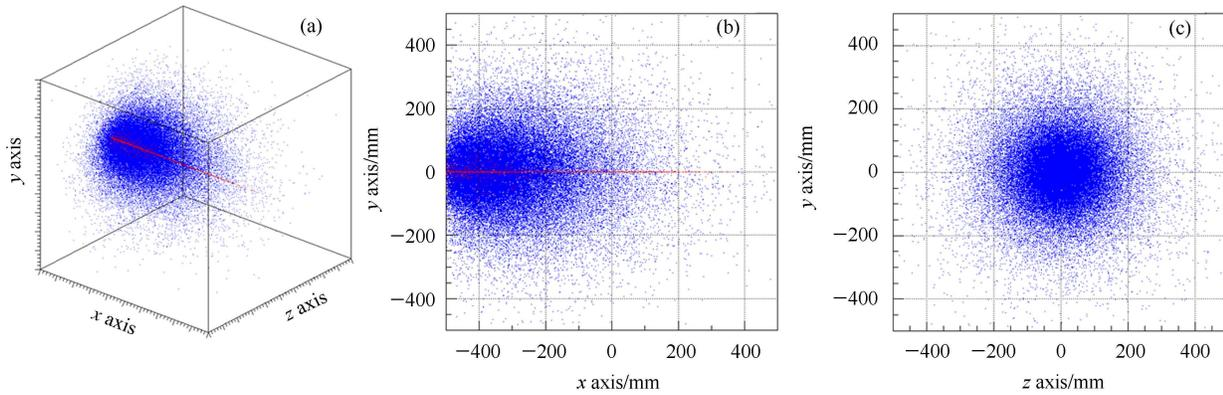
Fig. 4. (color online) Locations of neutron collision with proton first (Red) and Gd capturing (Blue).
