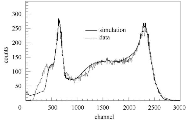
Fig. 1. Neutron spectrum captured by H and Gd when the Pu-C source is located at the center of the Gd-doped liquid scintillator prototype detector.
