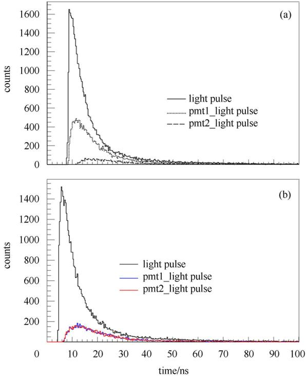
Fig. 10. (color online) (a) Waveforms of the light pulse drawn by recording photon generation in the scintillator and waveform of light pulses drawn by recording the photon number that arrived at each end of the detector when a neutron hit one end of the detector unit; (b) Waveforms of the light pulses drawn in the same way with (a) when a neutron hit the middle part of the detector unit.
