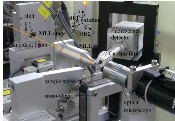
Fig. 4. The nano-focusing experiment system in beam-line 15U.
