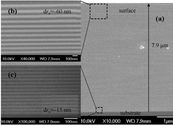
Fig. 3. SEM images of the cross-section of 7.9  $\mu\text{m}$ -MLL after the sampling process.
