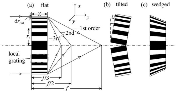
Fig. 1. A schematic of the MLL structure.
