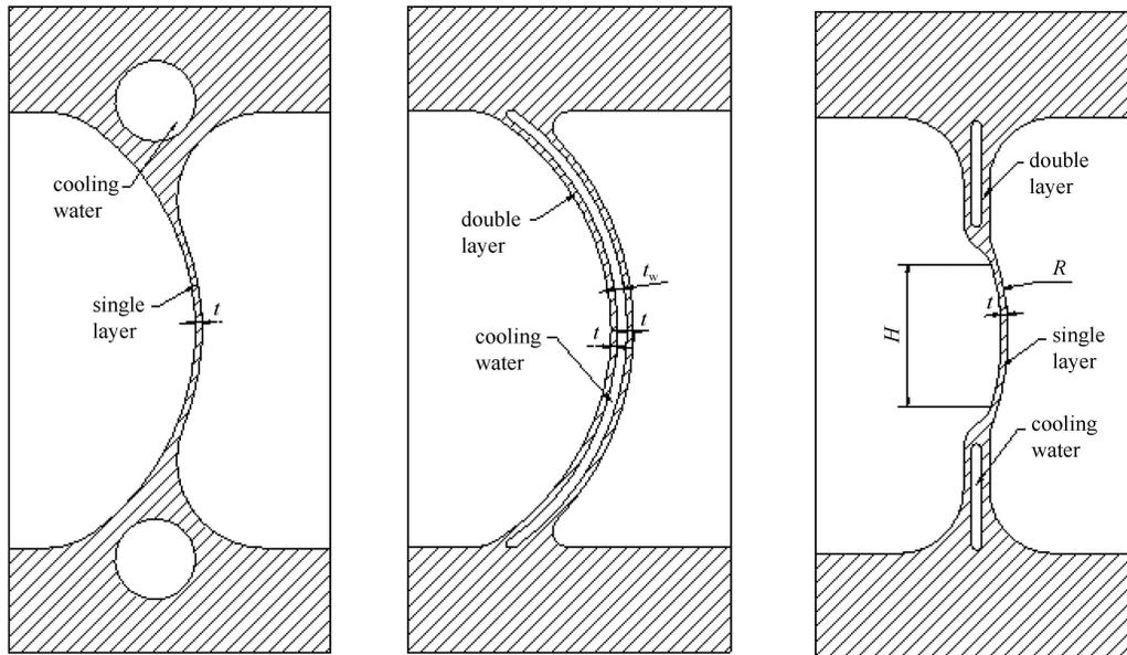
Fig. 2. The section views of three structures. (L: Single layer structure; M: Sandwiched structure; R: Single-double layer structure).
