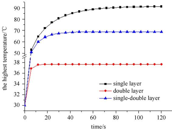
Fig. 3. Temperature comparison of cooling structures.
