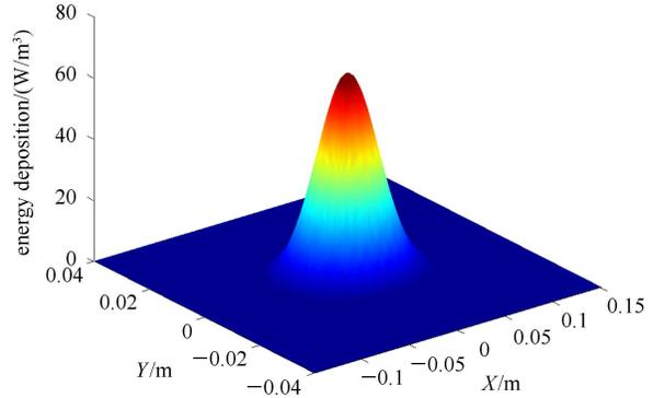
Fig. 1. Energy deposition distribution on a 2 mm thickness PBW.
