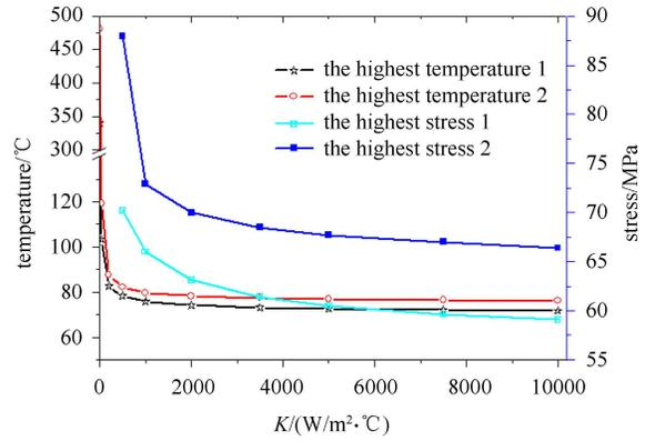
Fig. 9. The highest temperature and stress of the PBW vary with  $K$ . (1 denotes the values of  $K$  of two sides are equal, 2 denotes that of one side are 0).
