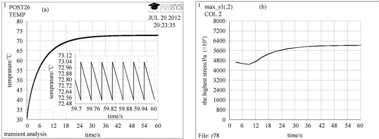
Fig. 7. The highest temperature and stress vary with time. (a) The highest temperature varies with time; (b) the highest Von Mises stress varies with time.
