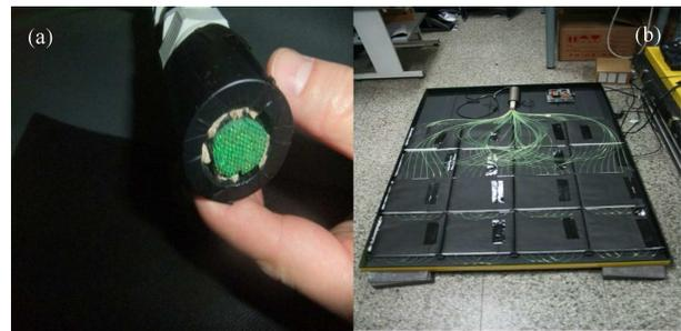
Fig. 10. (a)The fixing tube of WLS fibers; (b) the inner structure of ED box.
