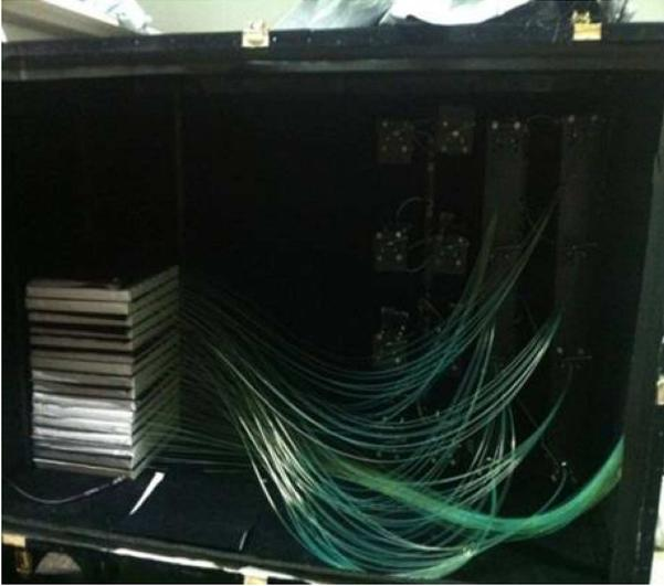
Fig. 7. The tile light yield test system.
