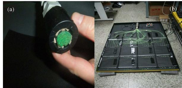
Fig. 10. (a)The fixing tube of WLS fibers; (b) the inner structure of ED box.
