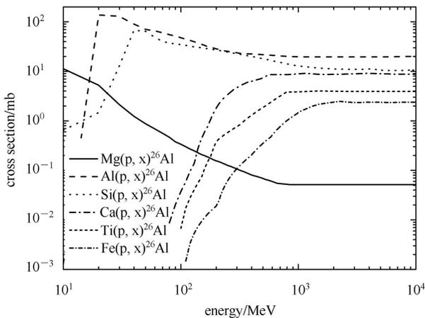
Fig. 3. The excitation function for proton induced reactions to produce  $^{26}\text{Al}$  on target elements Mg, Al, Si, Ca, Ti, Fe. These data are taken from Ref. [15].
