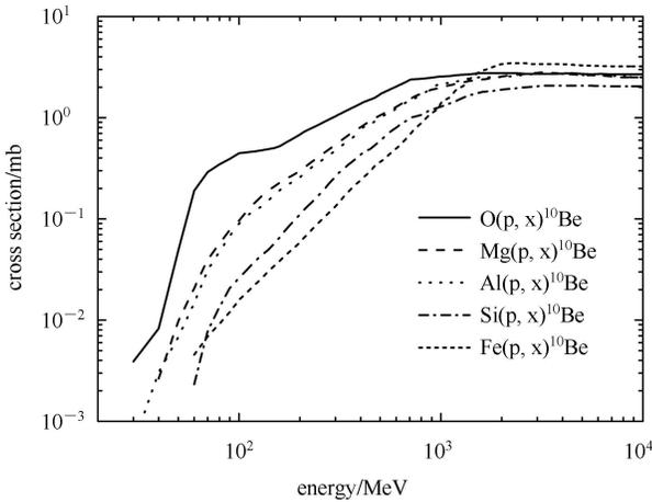
Fig. 2. The excitation function for proton induced reactions to produce  $^{10}\text{Be}$  on target elements O, Mg, Al, Si, Fe. These data are taken from Ref. [15].
