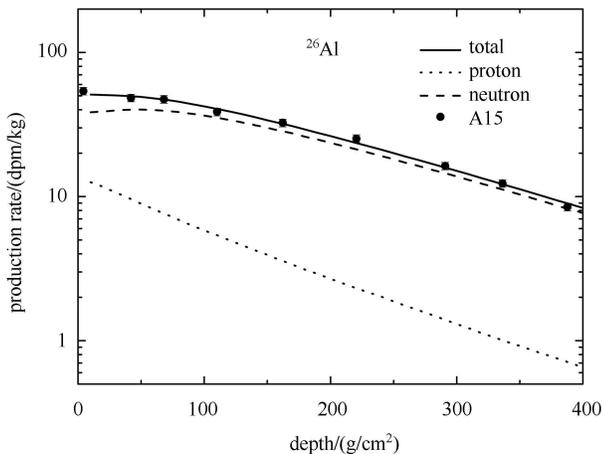
Fig. 6. The theoretical and experimental production rates of  $^{26}\text{Al}$  in the Apollo 15 drill core. The experimental data are taken from Ref. [18].
