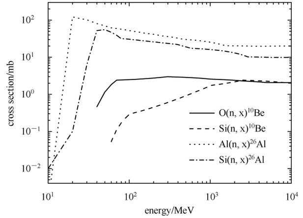
Fig. 4. The excitation function for neutron induced reactions to produce  $^{10}\text{Be}$  on target elements O, Si, and  $^{26}\text{Al}$  on elements Al, Si. These data are taken from Ref. [16].
