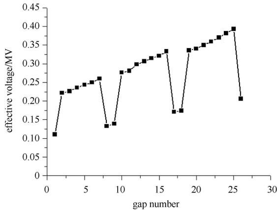
Fig. 7. The effective voltage in accelerating gap.
