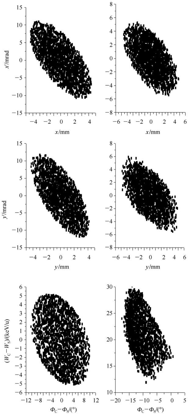
Fig. 2. Input particles distribution (100%) (left) and exit particles distribution (100%) (right).
