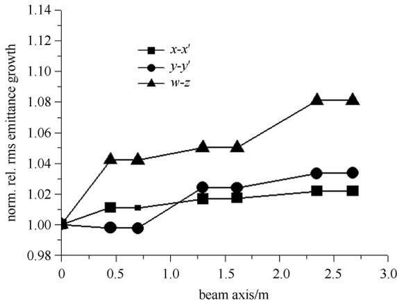
Fig. 5. Normalized RMS emittance growth.
