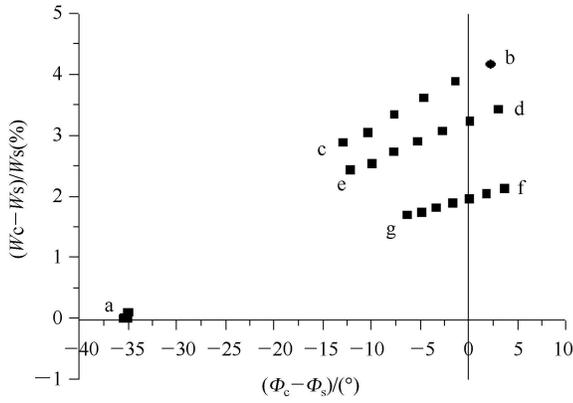
Fig. 3. The energy spread and synchronous phase at every accelerating gap (from ‘a’ to ‘g’).
