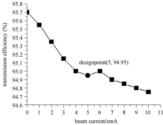
Fig. 6. Beam transmission efficiency.
