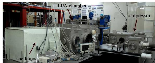
Fig. 5. Laser plasma experimental station.
