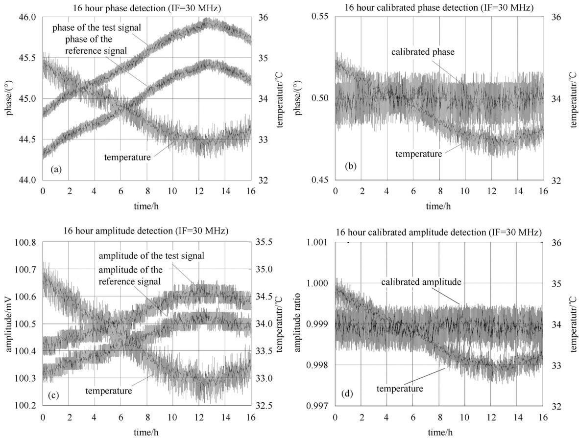
Fig. 8. Amplitude and phase detection of 30 MHz signal for 16 hours. (a) Phase detection before calibration. (b) Phase detection after calibration. (c) Amplitude detection before calibration. (d) Amplitude detection after calibration.
