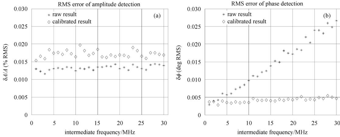
Fig. 7. The RMS errors of amplitude and phase versus different IFs before and after calibration.
