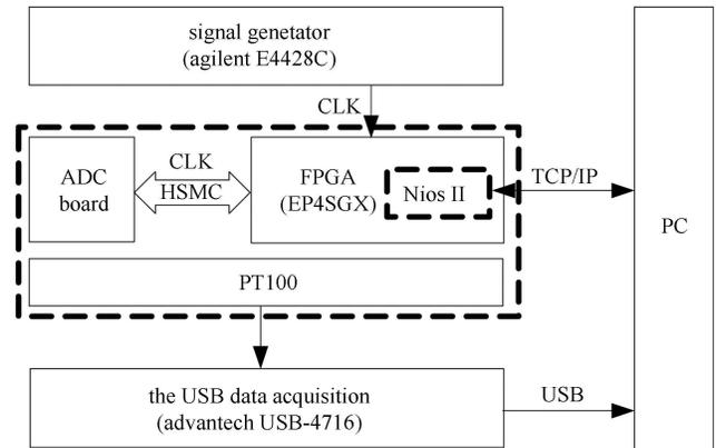
Fig. 6. Diagram of the experiment system.
