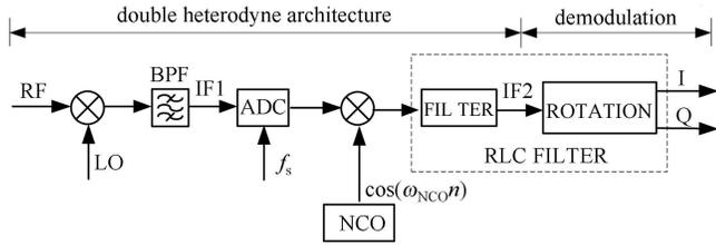
Fig. 2. A diagram of the proposed double heterodyne architecture.
