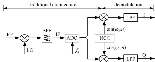
Fig. 1. Traditional IQ demodulation based on heterodyne architecture.
