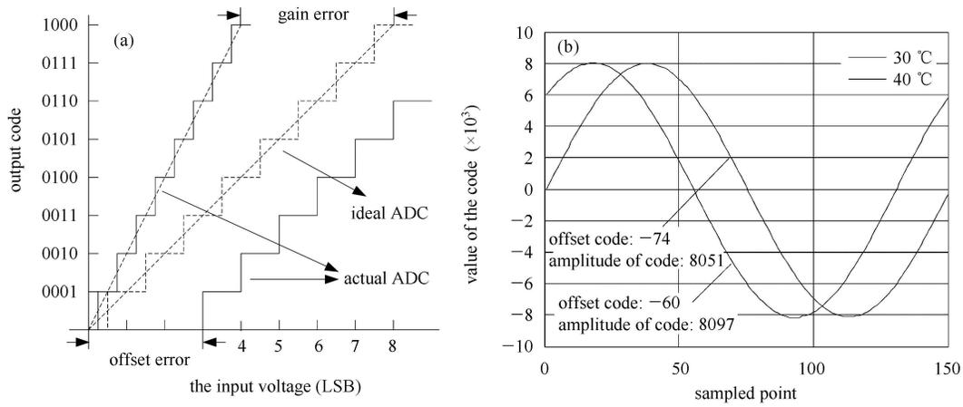
Fig. 5. Error analysis due to temperature variations and corresponding pointed solution. (a) Gain and offset errors. (b) Test of gain and offset error. A signal of 1 MHz has been sampled by AD9254 with 14-bit 150 Msp/s under different temperatures and recorded by a SignalTap II Logic Analyzer.
