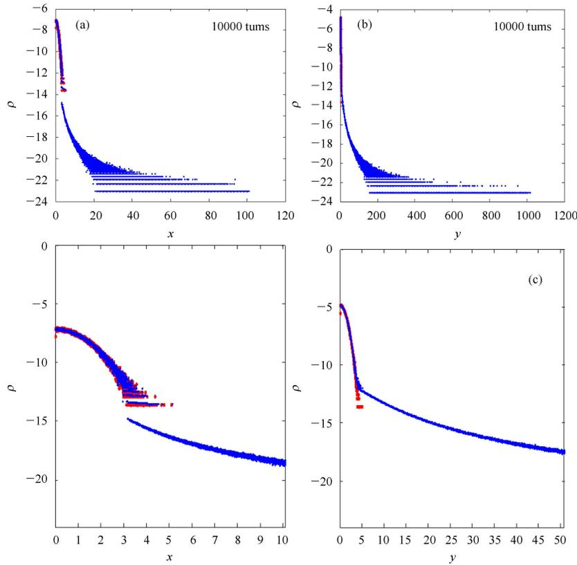
Fig. 8. The statistical distribution in transverse direction, the horizontal axis  $x/y$  is the distance normalized by the nominal horizontal/vertical beam size. The vertical axis represents the distributions in  $x/y$  using a logarithmic scale. The two pictures in (c) show the details in small distance.
