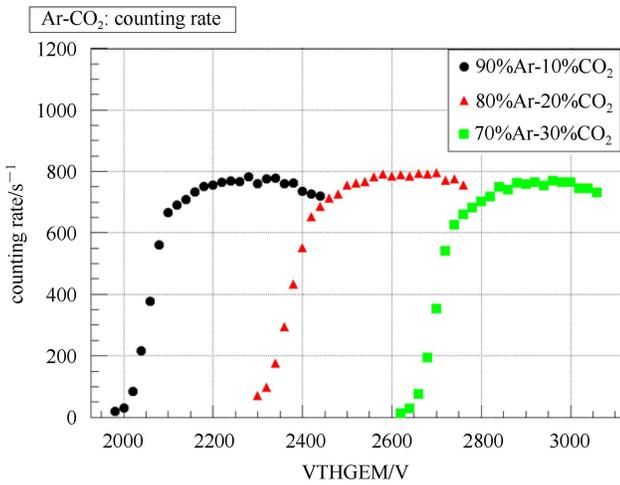
Fig. 4. Counting rate plateau with total HV.
