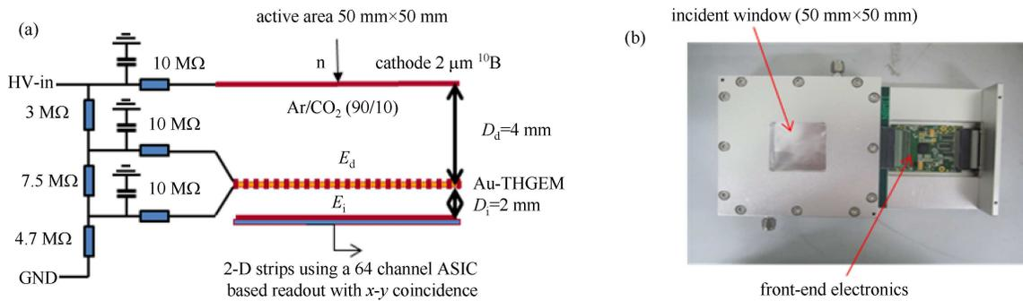
Fig. 1. Schematic of the detector prototype.
