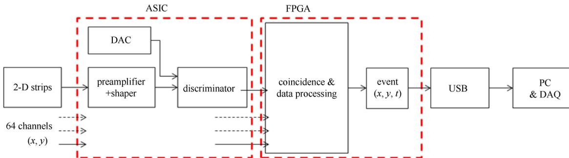
Fig. 2. Schematic of the data flow and processing.
