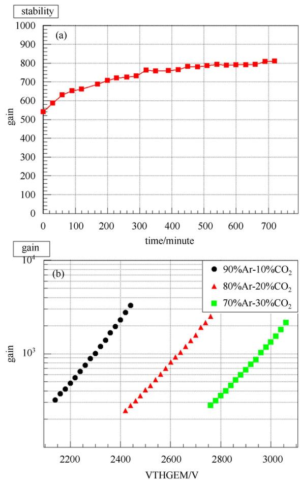
Fig. 3. Gain and stability of the THGEM.
