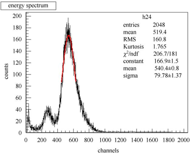
Fig. 5. A pulse height spectrum in the Ar/CO<sub>2</sub> (90%/10%) gas mixture.
