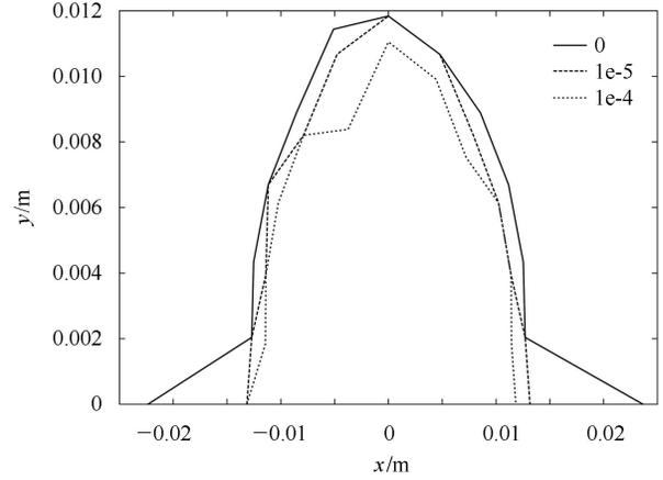
Fig. 3. Dynamic aperture of storage ring for different magnet errors (1024 turns, momentum offset is zero).
