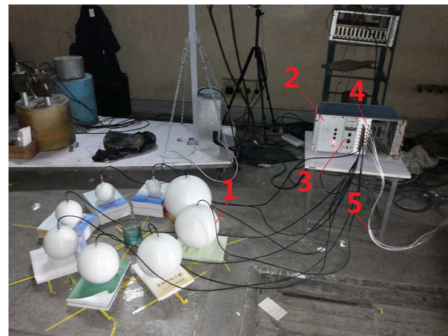
Fig. 1. (color online) The measurement environment of the ^{241}\text{Am-Be} neutron source. Part 1 is the high voltage and signal cable of the ^3\text{He} proportional counter in PS; Part 2 is a NIM chassis; Part 3 is the high voltage power supply module; Part 4 is the 8-channel pre-amplifier module in the NIM chassis; Part 5 is the output signal wires of the pre-amplifier which are pulled to the next-door monitoring room and connected to the main electronics system.
