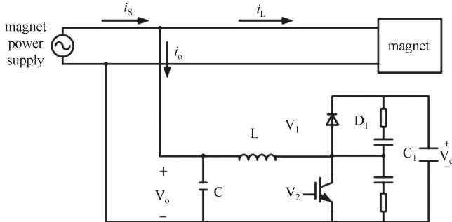
Fig. 3. APF working as a Boost circuit.
