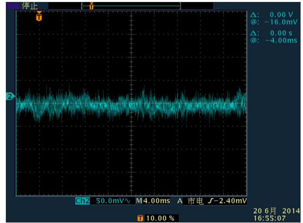
Fig. 13. (color online) Waveform of current ripple with APF connected, with MPS working at 40 A.
