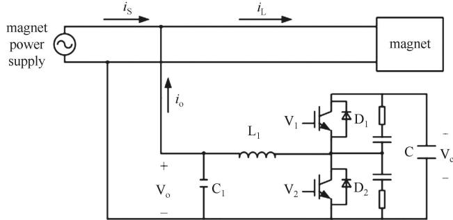
Fig. 2. Schematic of new APF topology.
