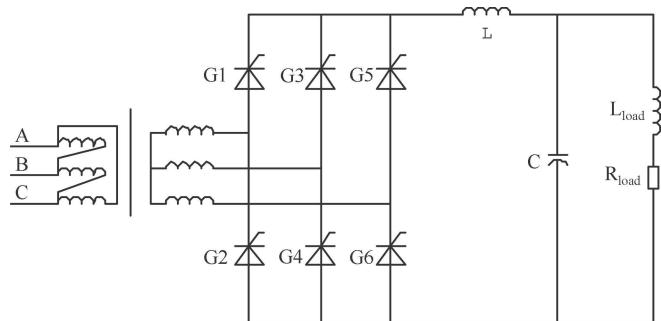
Fig. 7. Schematic of MPS prototype.
