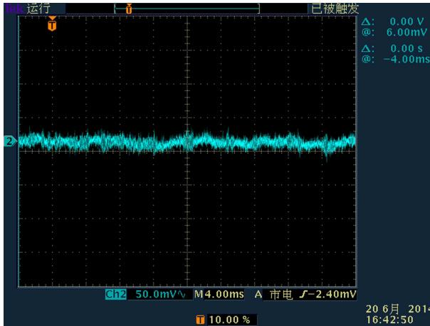
Fig. 11. (color online) Waveform of current ripple with APF connected, with MPS working at 24 A.
