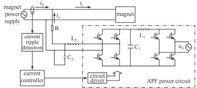
Fig. 1. Principle diagram of APF.
