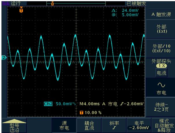
Fig. 10. (color online) Waveform of current ripple with MPS working at 24 A.
