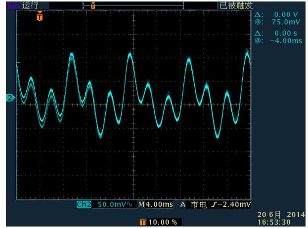
Fig. 12. (color online) Waveform of current ripple with MPS working at 40 A.
