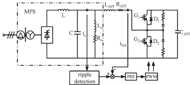
Fig. 5. Schematic of APF control loop.
