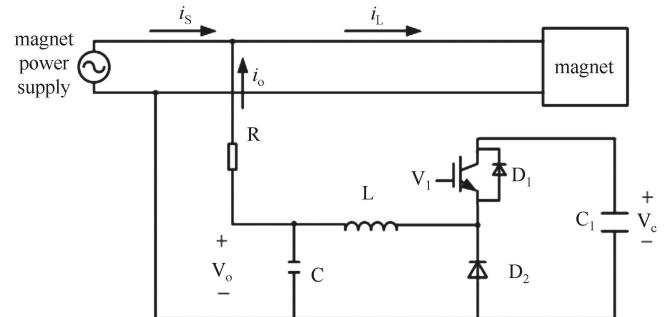
Fig. 4. APF working as a Buck circuit.
