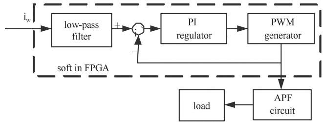
Fig. 8. APF control loop in FPGA.
